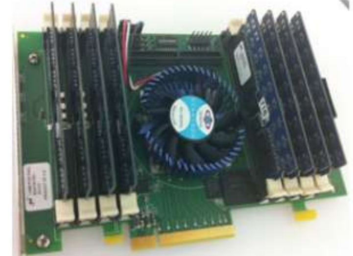
PCM SSD prototype
