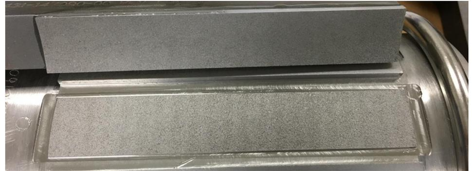
Example fracture surface in lever test
