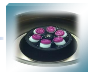
Centrifuging to remove unexfoliated particles
