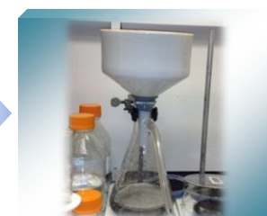
Filtration with PTFE filter
