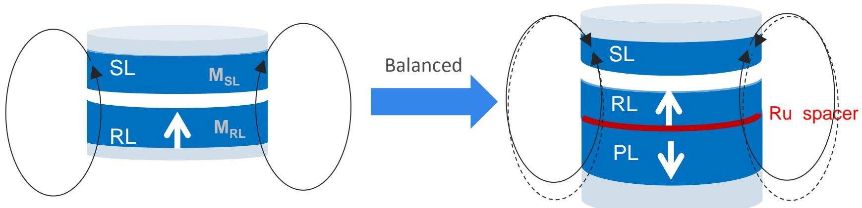
RKKY Oscillatory Coupling in non-magnetic spacer layer (**Ru**, Ir, Cr,...)
