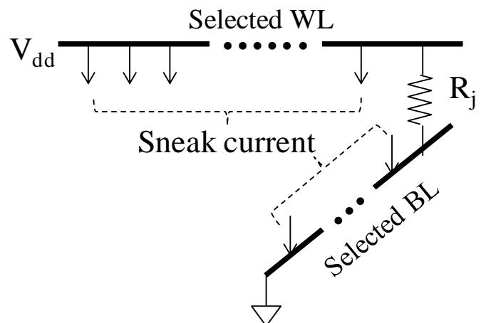
"1/3 bias": V drops to  $2V_{dd}/3$
