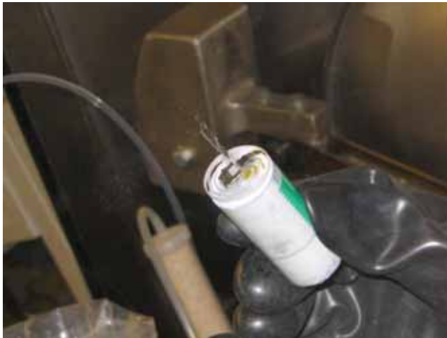
Cathode side of the jelly roll
