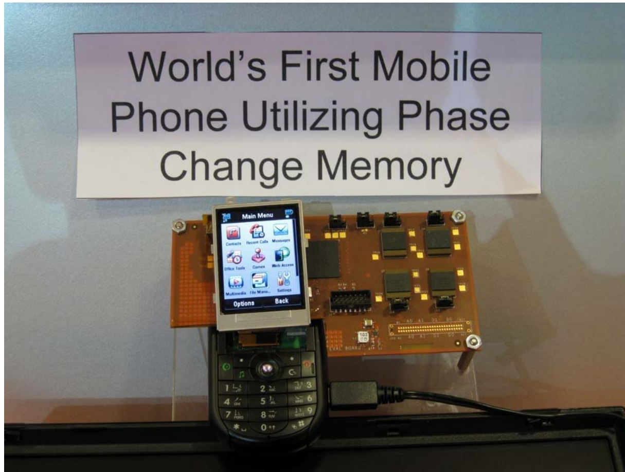
Intel and STMicroelectronics demonstration of a 128-Mbit, 90-nm phase-change memory in use with a mob phone to the Mobile World Congress at Barcelona, Spain. Reproduced from EE Times Europe, February 18, 2008
