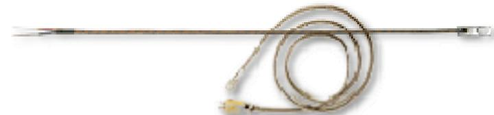
Temperature difference between two junctions can produce a voltage
