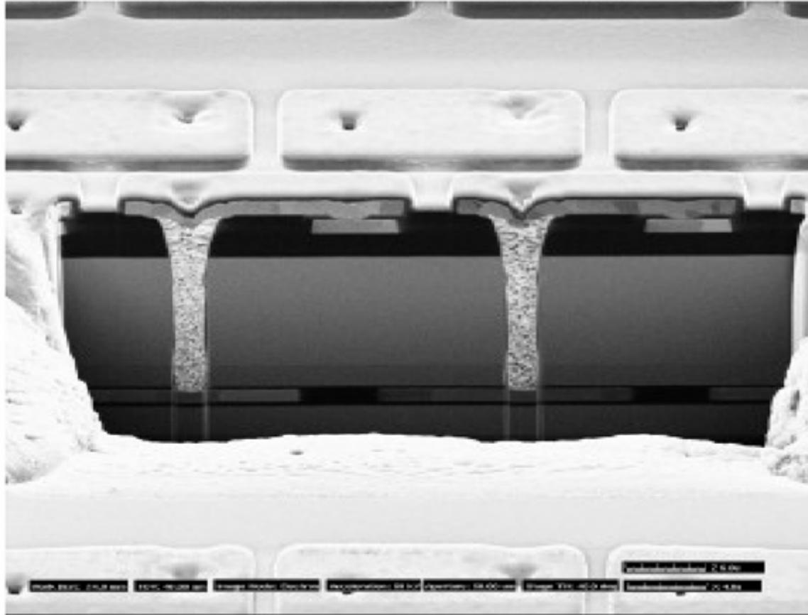
Cross section of a vertically integrated test chip structure, showing  $2.5 \times 2.5 \mu\text{m}^2$  interchip vias (FIB)
