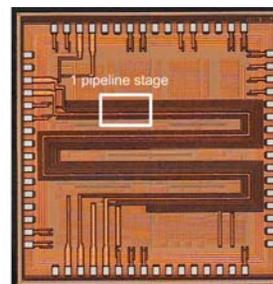
14-bit SiGe BiCMOS ADC chip layout & fabricated die
