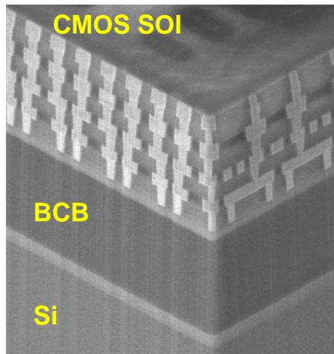
FIB image of bonded Freescale's 130nm CMOS SOI Cu/low-k wafer
