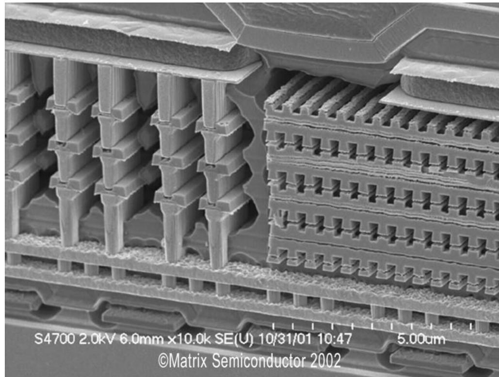
3D non-volatile memory (NVM) with polysilicon memory devices (Matrix Semiconductor)
