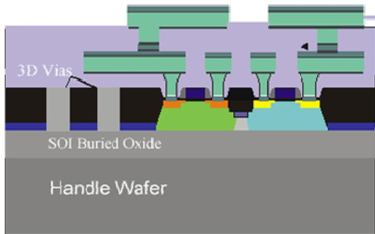
Photodetector layer: 10- $\mu\text{m}$  SOI CMOS
