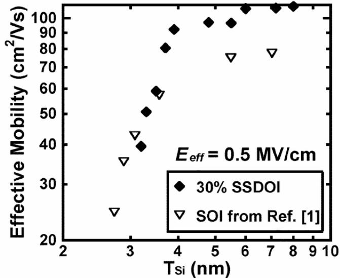
Fig. 3. Hole mobility for 30% SSDOI (this letter, solid symbols) and SOI (from [1], open symbols) at a vertical effective field of 0.5 MV/cm. At this field, the low dose channel implant in the SSDOI has limited influence on mobility [14]. Mobility for strained-Si decreases rapidly below  $T_{Si} = 3.9$  nm, possibly due to thickness-fluctuation-induced scattering, as observed for ultrathin unstrained SOI in [1] and [4].
