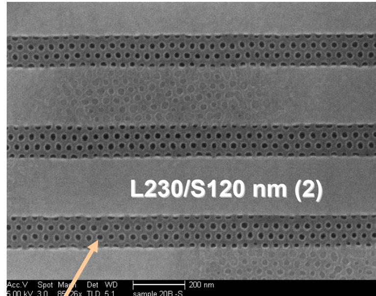
Self-aligned nanoscale contact holes using diblock copolymer self-assembly
