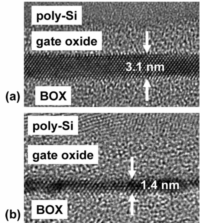
Fig. 1. XTEMs of (a) 3.1-nm-thick 40% SSDOI, and (b) 1.4-nm-thick 30% SSDOI.  $C-V$  measurements confirmed the continuity of the film.
