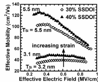
Fig. 4. Hole mobility versus effective electric field for 30% SSDOI (open symbols) and 40% SSDOI (solid symbols). Even for  $T_{Si} = 3.1$  nm, mobility increases as the strain in the Si is increased. Locally thinned MOSFETs were used for this comparison.
