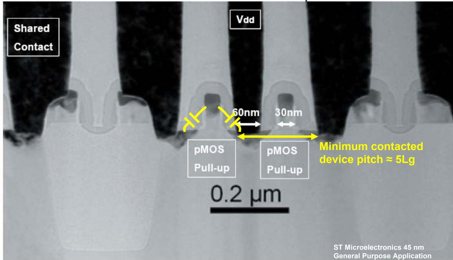
Fig. 12 : TEM cross section inside a  $0.334\mu\text{m}^2$  6T-SRAM bit-cell
