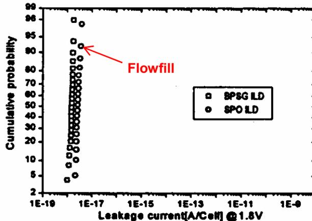
Leakage current between bit line and top electrode
