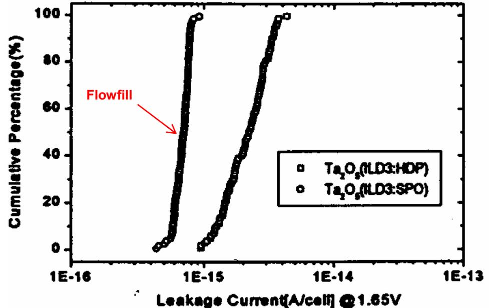
Leakage current of Ta<sub>2</sub>O<sub>5</sub> capacitors for HDP and Flowfill
