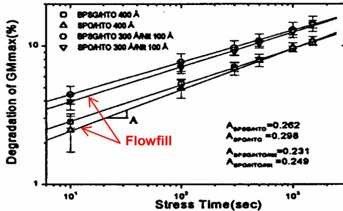
Degradation of  $G_{m_{max}}$  in NMOS as a function of hot carrier stress time. ( $W/L=10/0.3\mu m$ ,  $V_G=1.38V$ ,  $V_D=3.25V$ )
