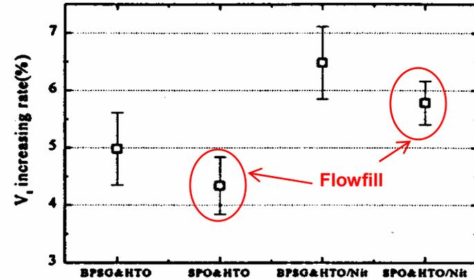
Variation of threshold voltage in PMOS after BT stress ( $W/L=10/0.4\mu m$ ,  $V_G=-6.5V$ ,  $200^\circ C$ , 10min)
