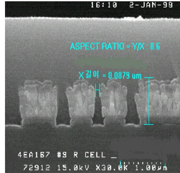
(b) Space  $0.09\mu\text{m}$ , AR 8.6:1(negative sloped pattern)
