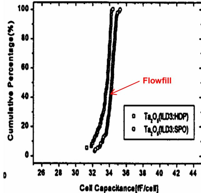
Capacitance of Ta<sub>2</sub>O<sub>5</sub> capacitors for HDP and Flowfill
