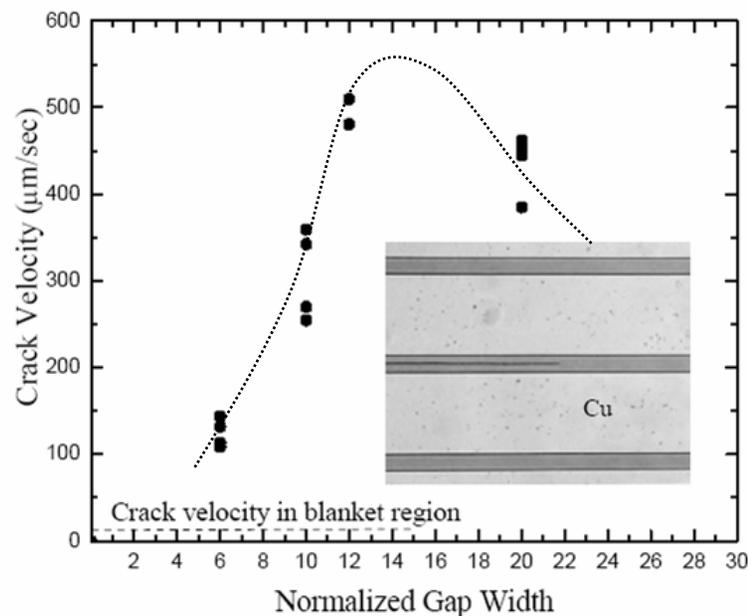
Crack velocity measured at various gap widths. The insert shows a channeling crack in a 3  $\mu\text{m}$  thick dielectric overlayer induced by the presence of a gap between two wide copper plates.
