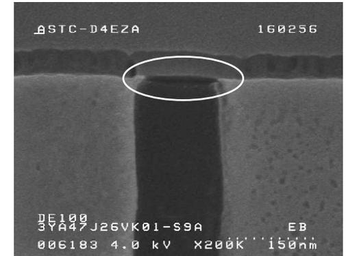
Severe Erosion at CMP
