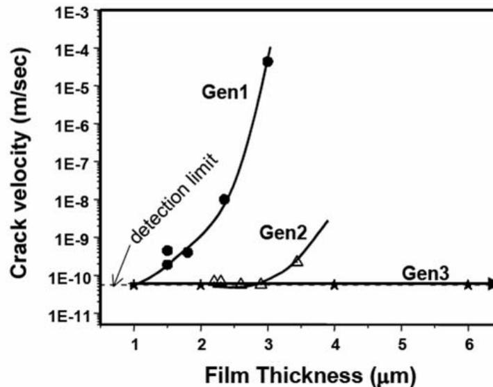
Crack development velocity at 100% humidity
