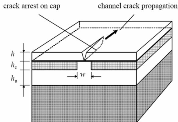
Multi-layer structure of underlying patterned metal and dielectric layers with a channeling crack in the overlayer.
