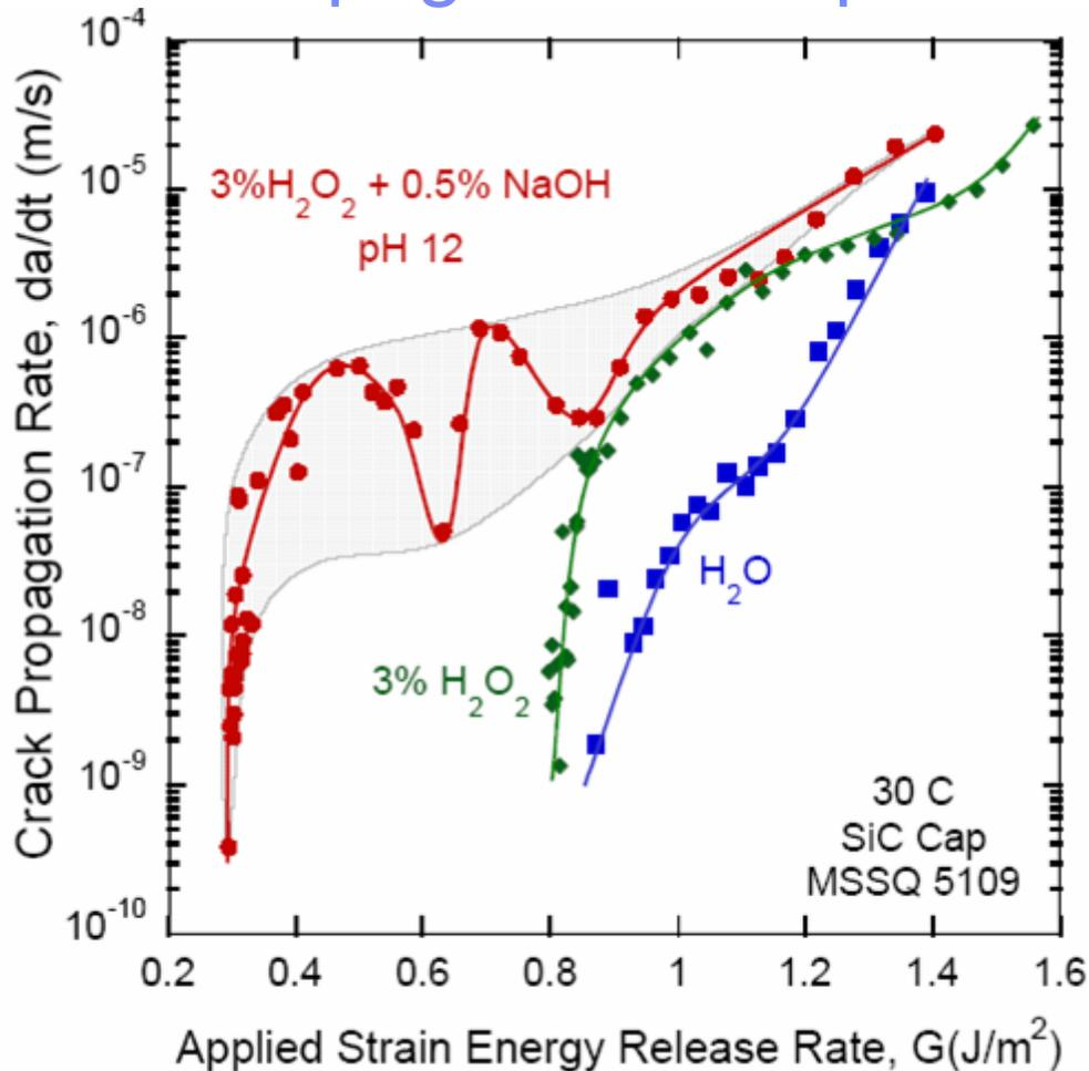
The corrosion of MSSQ in  $\text{H}_2\text{O}_2$  + NaOH solutions allows cracking to extend to extremely low values of  $G$ .
