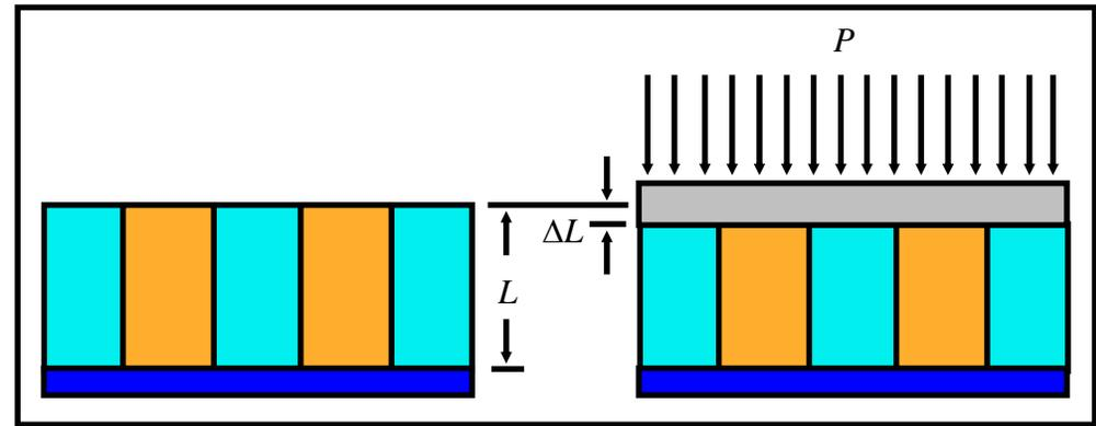
$$\sigma_{\text{Cu}} = P \left( \frac{E_{\text{Cu}}}{pE_{\text{Cu}} + (1-p)E_{\text{diel}}} \right)$$
