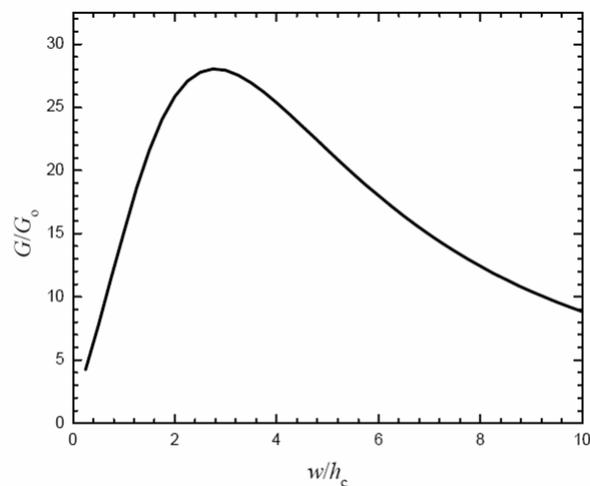
Energy release rate versus the gap width between metal pad
