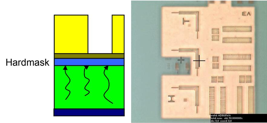
ARC/Photoresist applied onto oxide hardmask over SiCOH (K=3) dielectric – images develop properly
