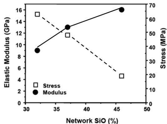
Elastic modulus and stress of SiCOH films vs. fraction of network oxide.
