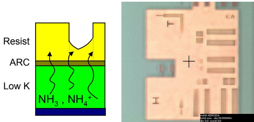
ARC/Photoresist applied directly onto SiCOH (K=3) dielectric – images fail to develop properly
