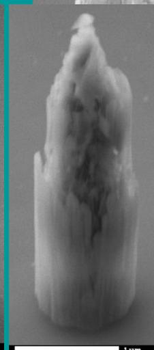
Oxidation proceeds by roughing the surface and generation of cavities
