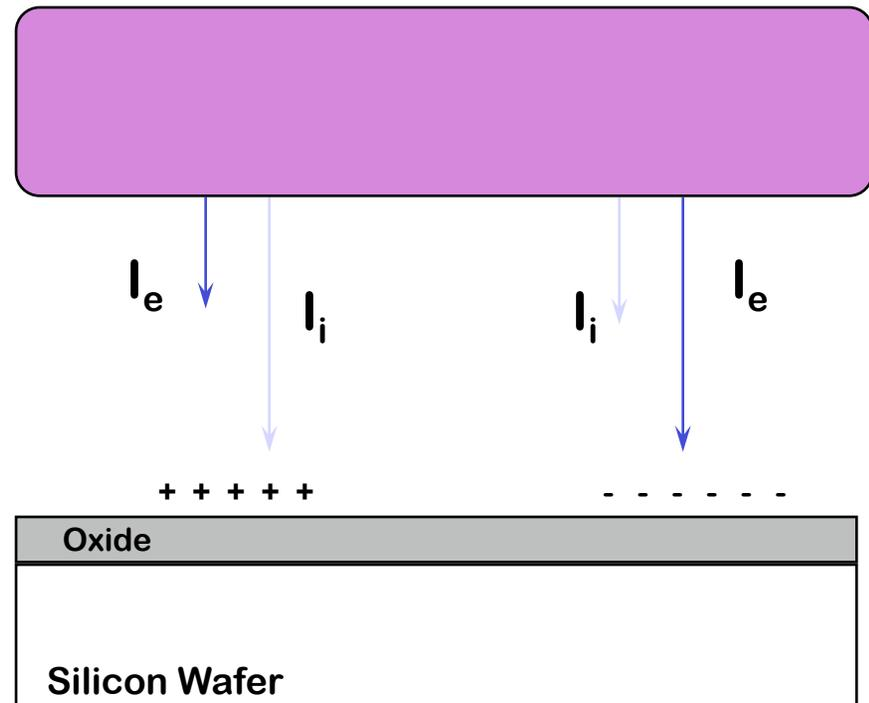
Recommended Oxide thickness >1000A
