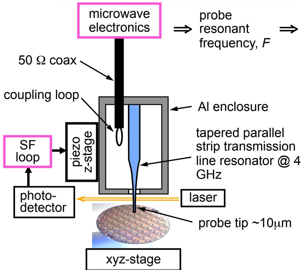
microwave electronics  $\Rightarrow$  probe resonant frequency,  $F$   $\Rightarrow$
