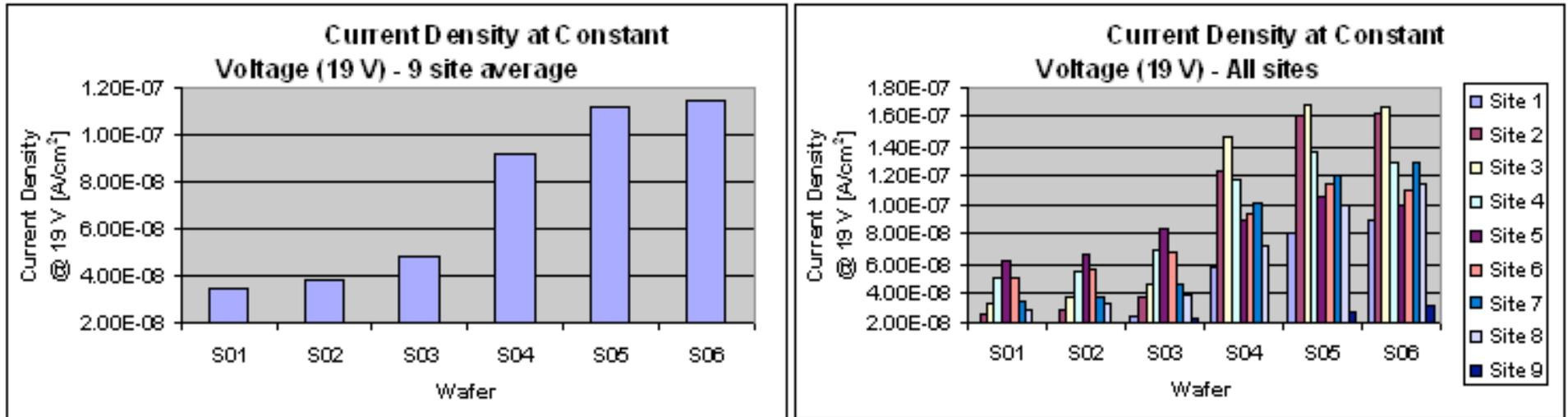
Chamber 1 & 2 were the same type / same manufacturer. The film was PMD (pre-metal dielectric), and device data from chamber 2 was showing higher leakage characteristics than from chamber 1.
