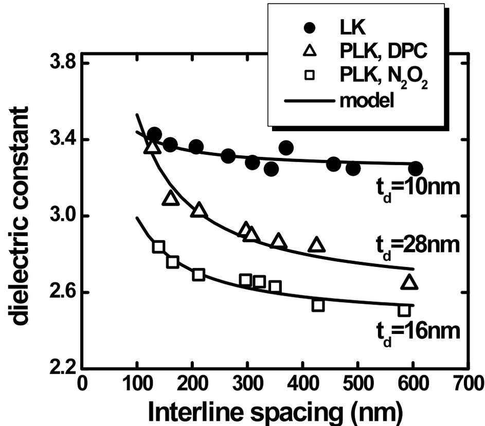
Dielectric constant of remaining after etch low- $k$  dielectric extracted from experimental data for non-porous (LK) and porous (PLK) low- $k$  materials. Solid lines are the fits to an analytical model for sidewall damage contribution. LK exhibits minimal processing induced damage, while PLK damage depends on processing. Dry preclean induces more damage than N<sub>2</sub>O<sub>2</sub> ash.
