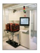
Complex Force measurement load-cell, both measuring and correcting for internal and external forces which affect weight measurement 127.6730 –
