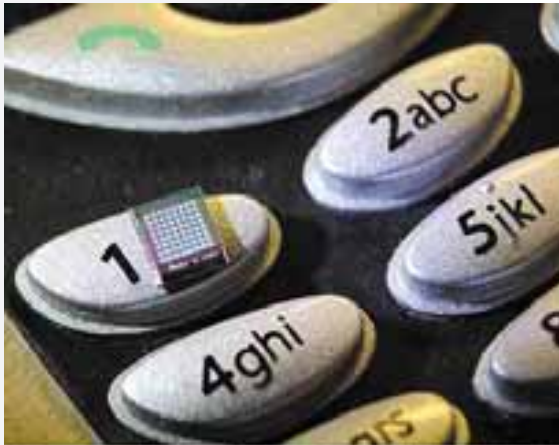
Big performance from a small, low-cost chip is the claim to fame of this multielement MEMS IC with an onboard amplifier. Produced by Akustica, it heralds the next technological revolution in acoustics for the hearing impaired and for cell phones.
