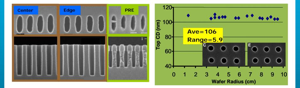
Comparing with pre mask surface roughness and mask open cross section, an improved contact hole distortion with a very decent profile was obtained with adding PDP for 20sec before BARC open
