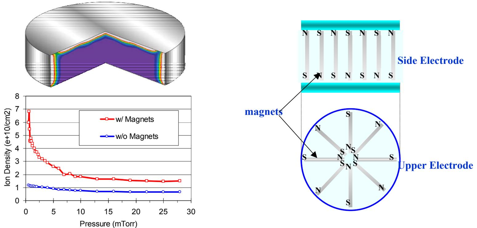
Permanent SmCo magnets are embedded in the upper and sidewall electrodes; alternating poles faces creates magnetic fields that reflects electrons back into the plasma volume.
