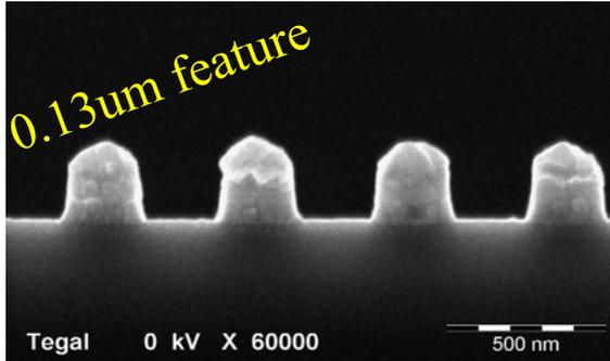
The combination of Dual Frequency HRe<sup>-</sup> with High Temperature ESC results in enhanced etch capability to the 0.13 micron device node.
