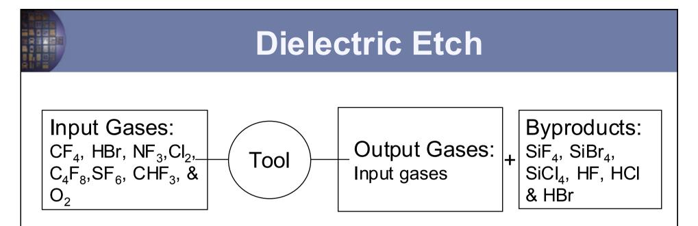
•Safety:  $Cl_2$  is toxic (TLV=1 ppm) and an irritant; byproducts are acidic with TLVs levels below 5 ppm. SiX<sub>4</sub> will block ducts, generate HX (X = F, Cl, Br)
