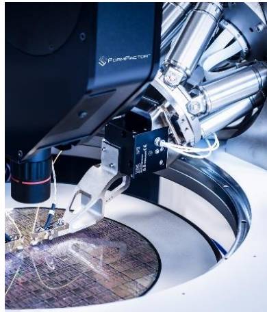
6-Axis/Piezoelectric Positioner, Single Fiber/Fiber Array, Displacement Sensors
