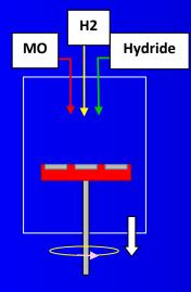
Vendor - A • Turbo-Disk; MO + Hydride • 3-inch x 24 Wafer Capacity
