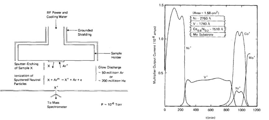
Ion sputtering and detection of composition in gas phase
