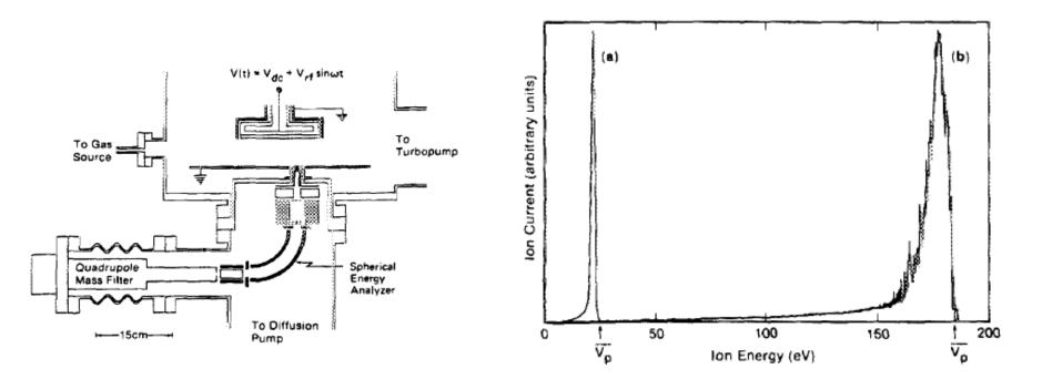
Coupling ion energy measurements with understanding plasma electrical behavior
