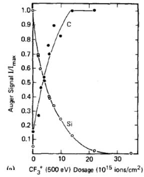
It is suspected that the deposition and removal of carbon is one of the most important phenomena affecting the operating characteristics of plasma-etching systems.
