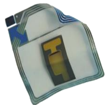
IPS "Thinergy" TFμB on Cu/Ni foil
