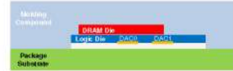
Figure 3. Side view of a DRAM die on top of a logic die
