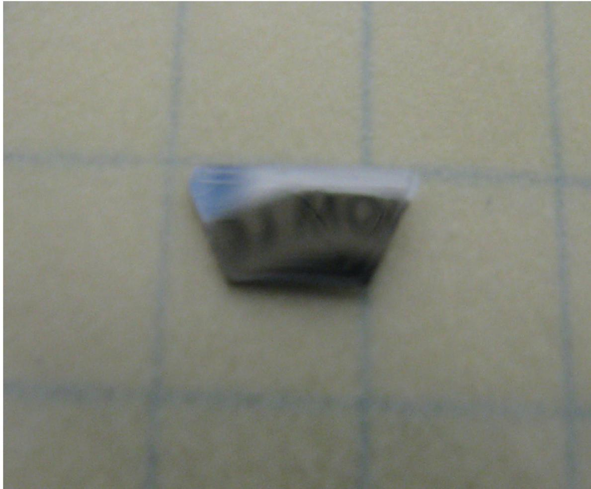
**Flat crystal: ~7.4mm long; area ~ 0.18cm<sup>2</sup>; ~75μm thick; grid lines 0.25" apart.**
