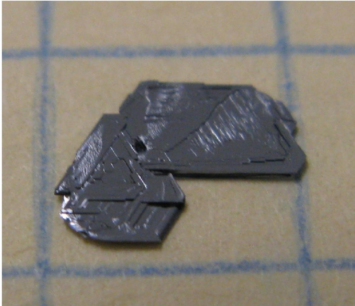
**Flat bicrystal: ~7.0mm long; area ~ 0.26cm<sup>2</sup>; ~96μm thick.**
