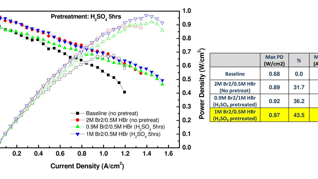
prmance from <u>pretreated</u> PM with H<sub>2</sub>SO<sub>4</sub> was very reliable ix power : 0.92 (0.9M Br2/1M HBr) and <u>0.97</u> (1M Br2/0.5M HBr) ix current density: 1.54 A/cm2
