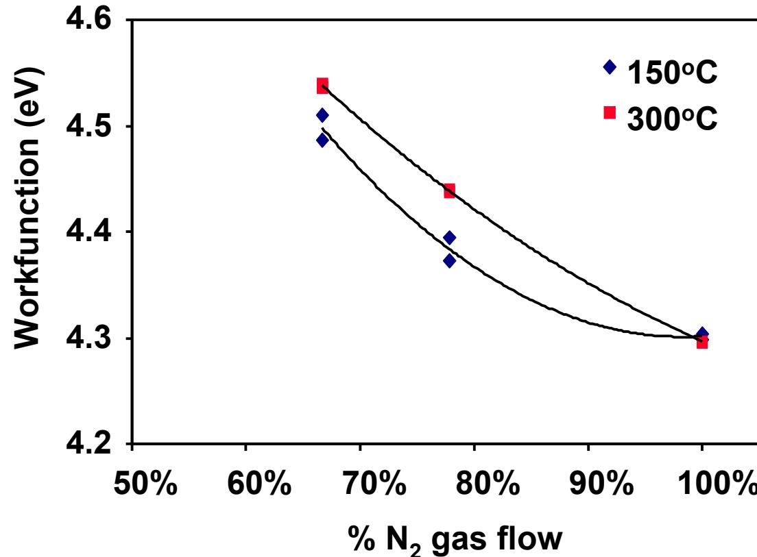
N<sub>2</sub>/Ar flow ratio during reactive sputter deposition of TiN
