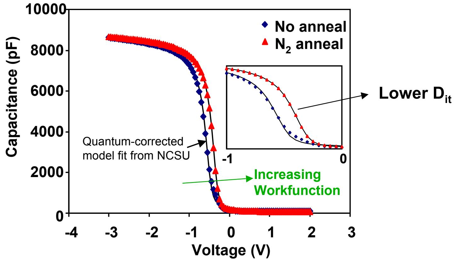
Sub-atmospheric  $N_2$  anneal increases workfunction and should improve reliability of TiN metal gate transistors
