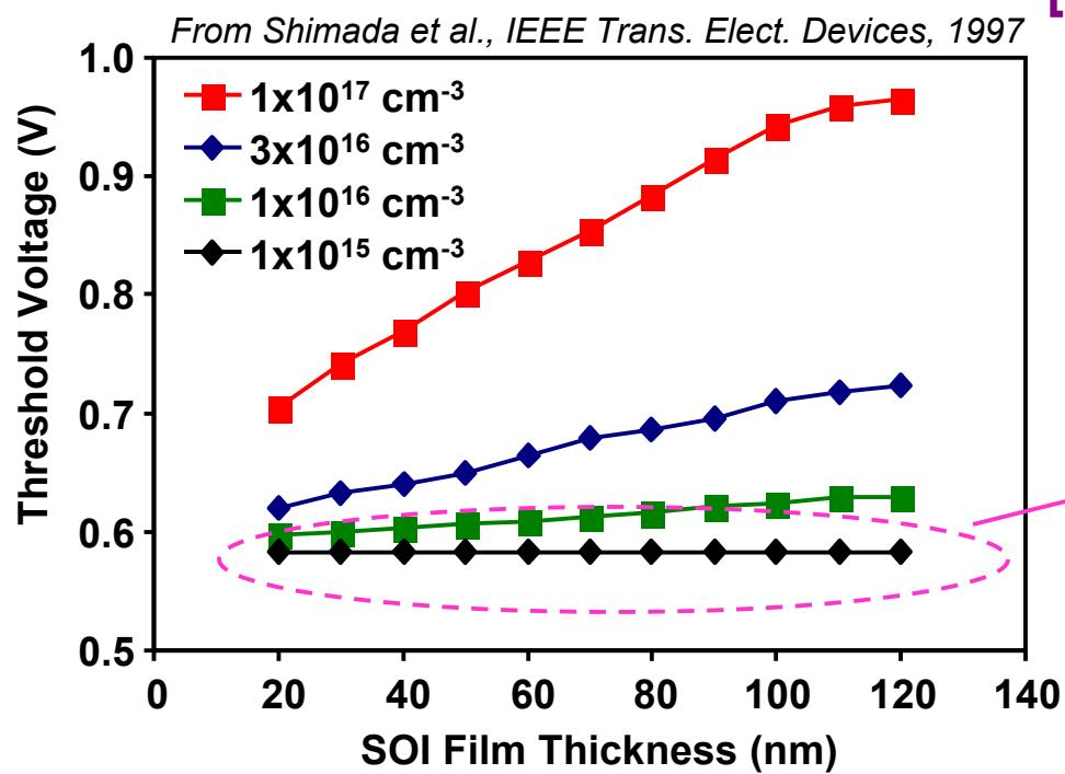
Low channel doping reduces  $V_t$  variation, critical for subthreshold operation
