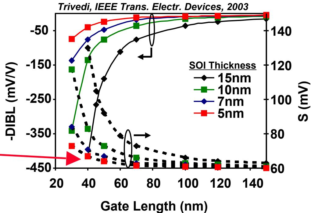
Below 40nm, non-planar SOI designs may be necessary for improved channel control
