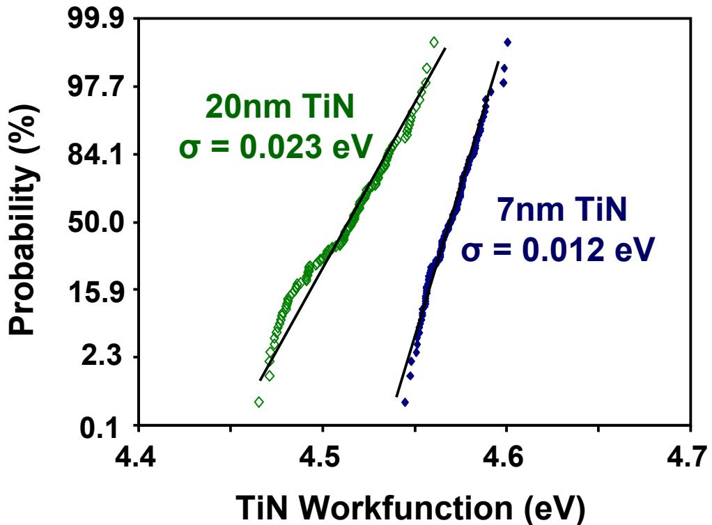
Reducing TiN thickness: 1) increases workfunction,
