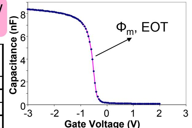
C-V curves fit using quantum corrected model from NCSU<sup>1</sup>
