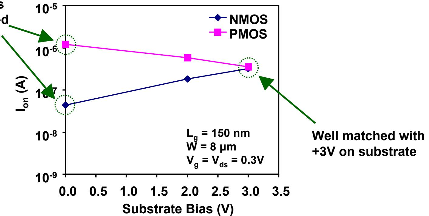
SOI transistor design enables use of substrate biasing to match NMOS and PMOS transistors in subthreshold operation
