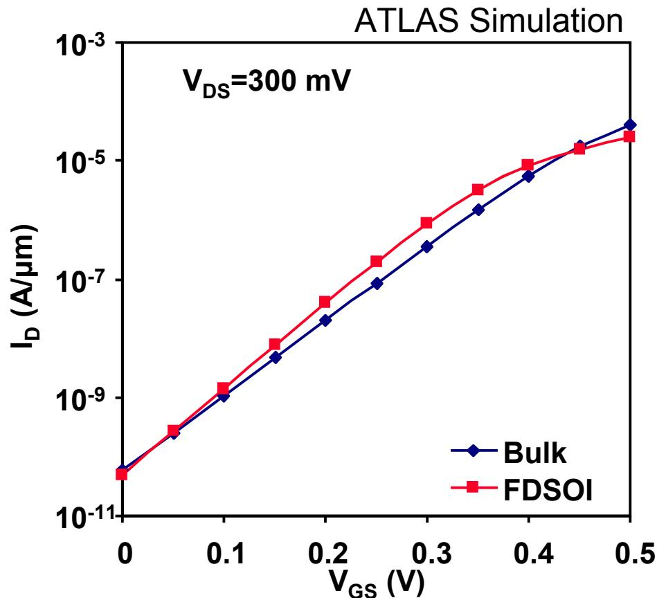
FDSOI exhibits 2.5x improvement in  $I_{on}/I_{off}$  ratio at 0.3 V
