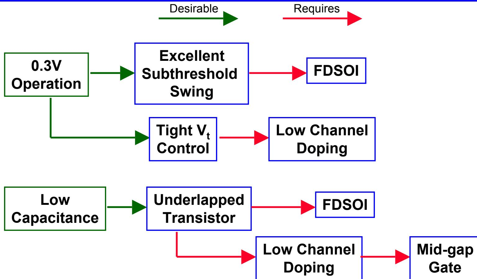
The improved ULP transistor will have four key components:
