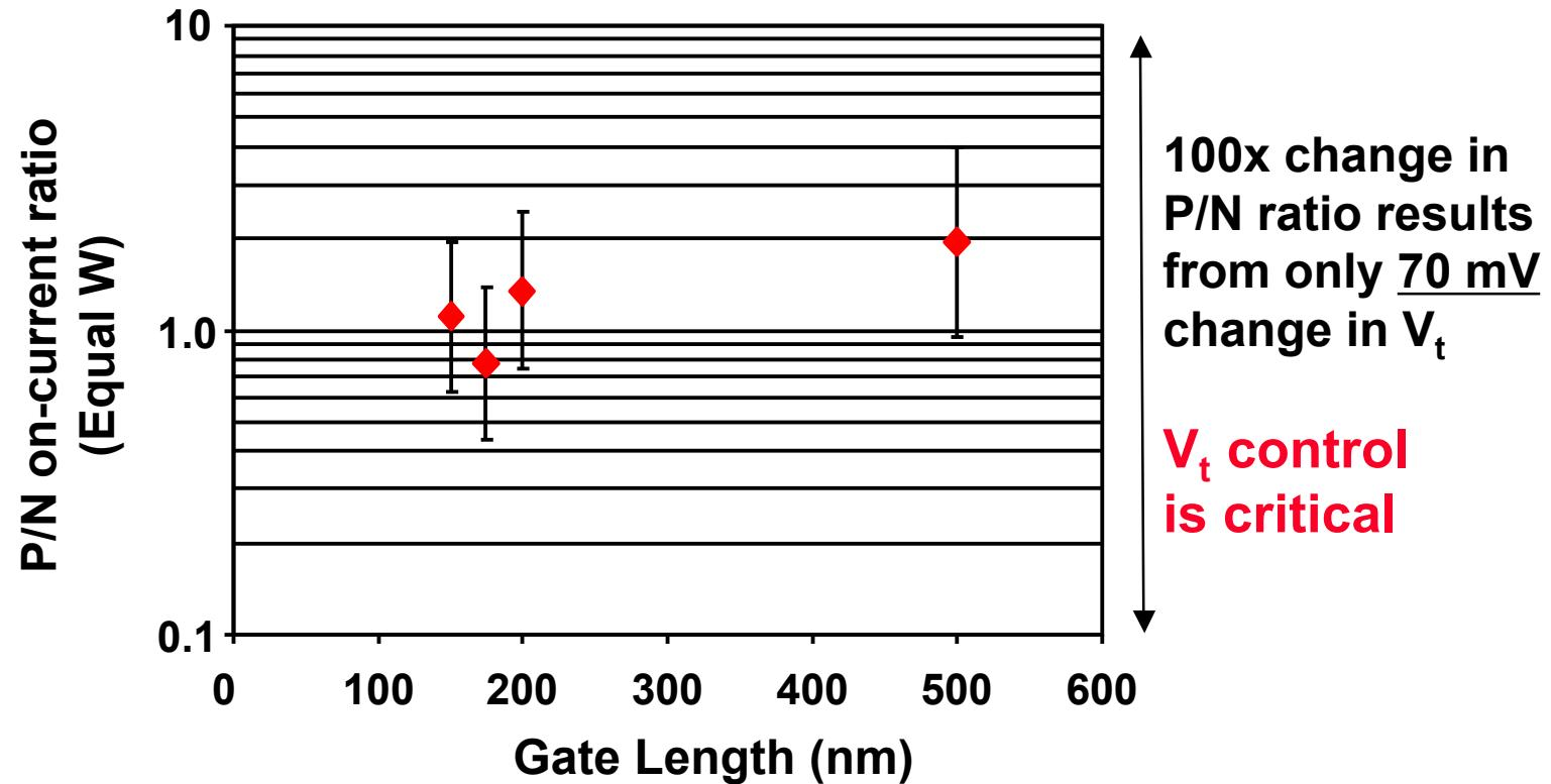
Equal  $I_{on}$  allows equal NMOS and PMOS transistor sizing and equal N and P device capacitance
