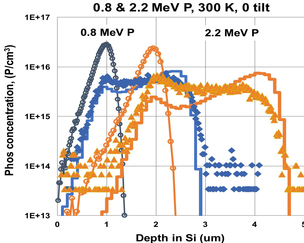
0.8 and 2.2 MeV Phosphorous channelled profiles, SIMS (symbols), IMSIL (histograms), TRIM (open circles, amorphous Si). Dose =  $1\text{e}12 \text{ P}/\text{cm}^2$ .
