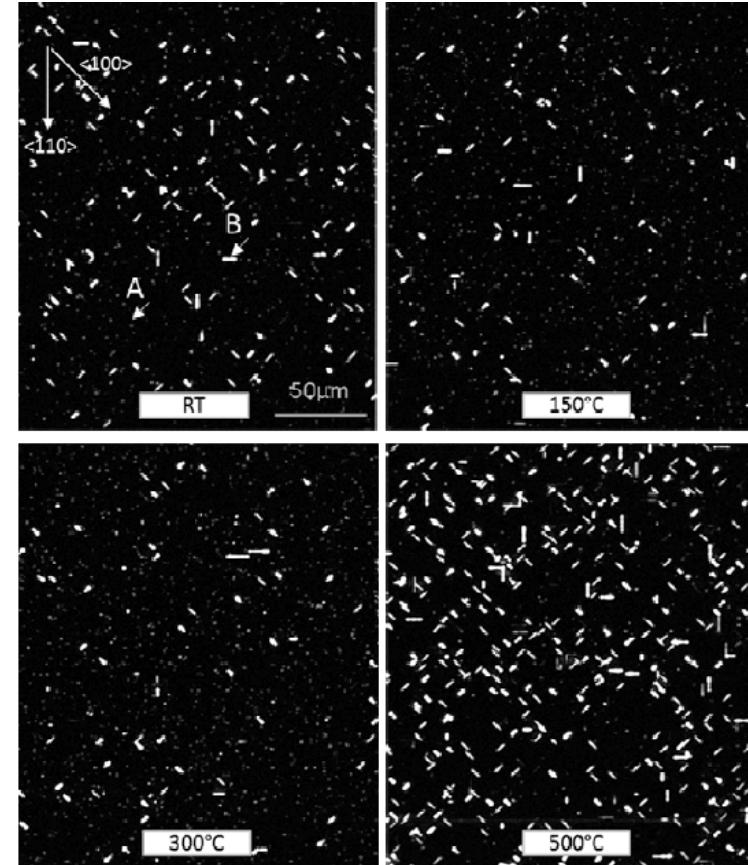
Fig. 4. PL results on Phosphorus  $6\text{E}13 \text{ at/cm}^2$  after anneal at  $950^\circ\text{C}$  N<sub>2</sub>/O<sub>2</sub> (5%) 3min. Radiative dot and elongated defects are exhibited. Arrow A defined a dot defect, arrow B defined an elongated defect.
