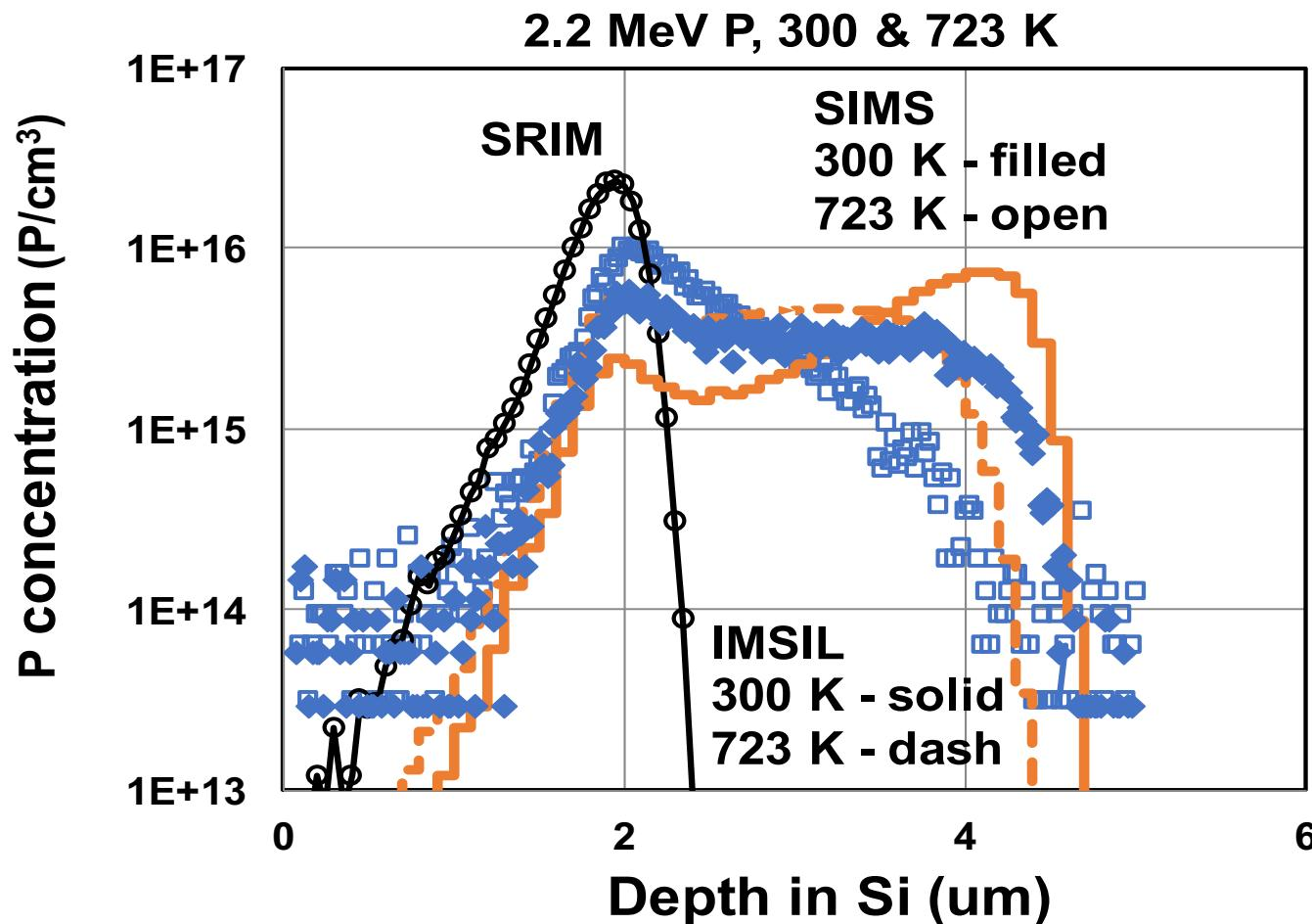
2.2 MeV Phosphorous channelled profiles at wafer temperatures of 300 and 723 K,
