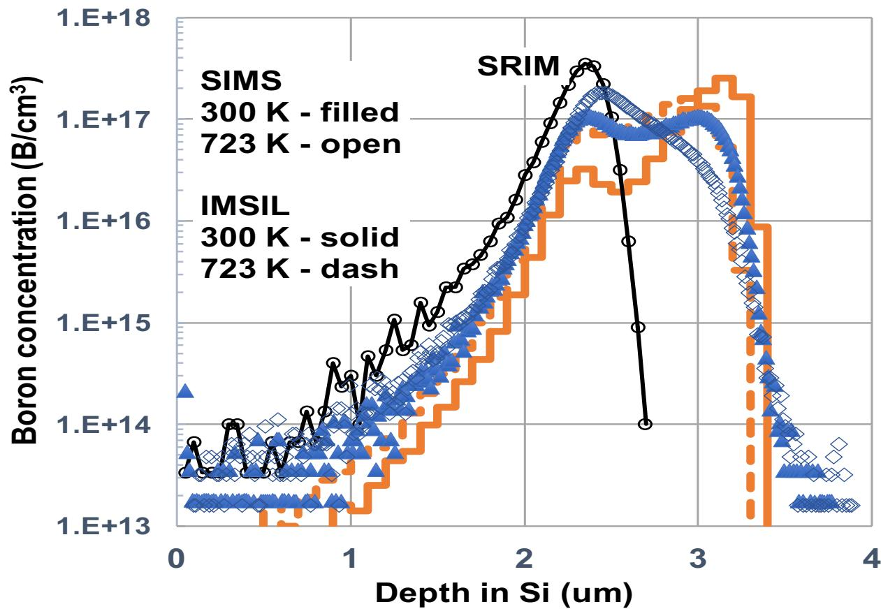
1.5 MeV Boron channeled profiles at wafer temperatures of 300 and 723 K, **SIMS (symbols)**, **IMSil (histograms)** and **SRIM (open circles)** for amorphous Si target (no channeling). Dose =  $1\text{e}13 \text{ B}/\text{cm}^2$ .
