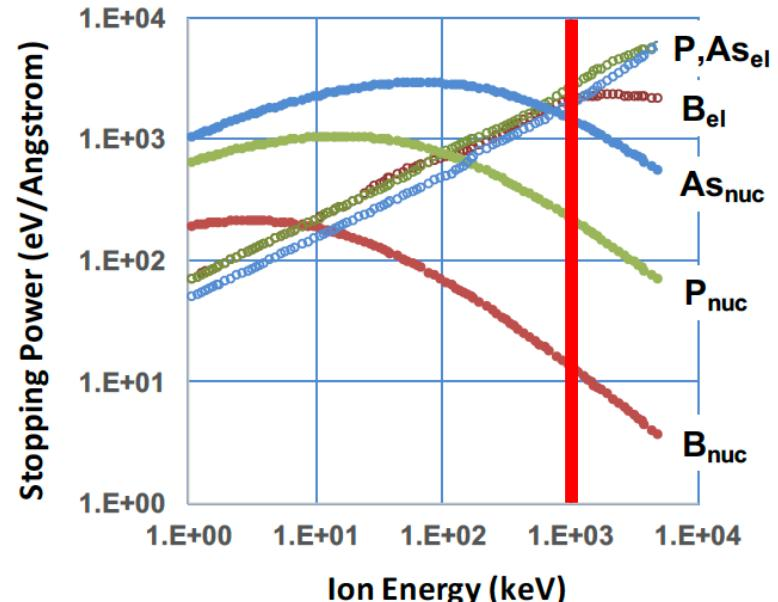
For MeV B,  $S_{nuc}$  is  $\approx 1\%$  of total stopping, weak channeling impact on range.
