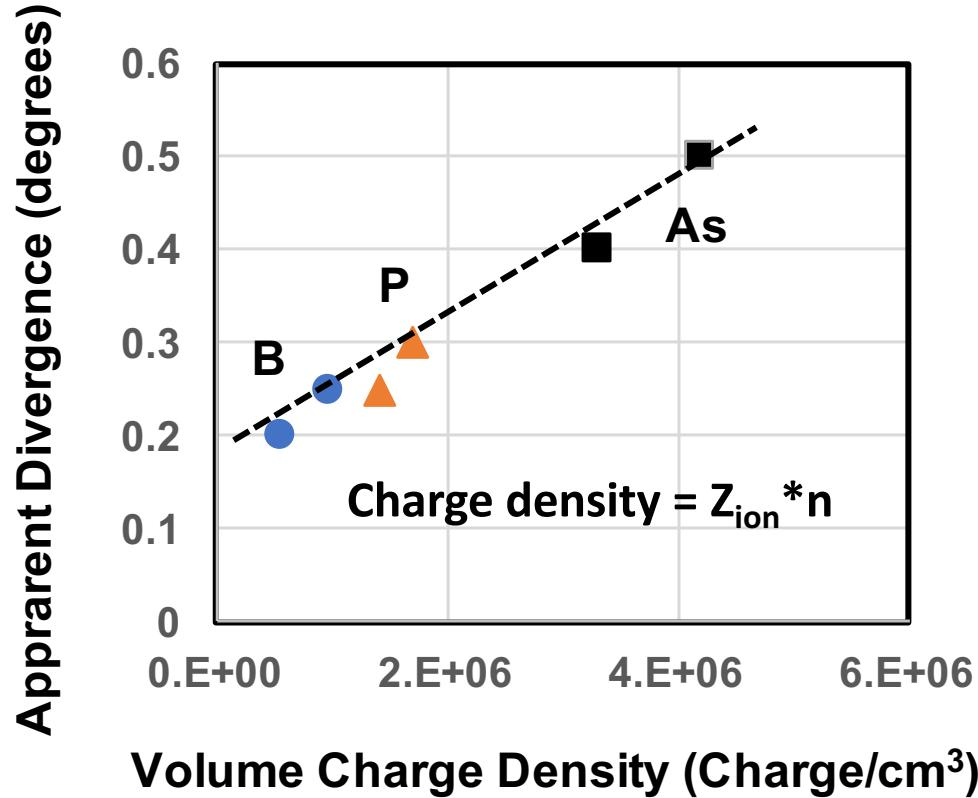
Apparent ion beam divergence angles, as judged by channeled profile shape and location, for B, P and As ions in the energy range of 0.8 to 3.1 MeV.
