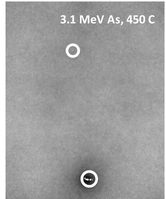
PL-imaged defects at a depth of  $\approx 5$  um over a 175x140 um field of view for annealed 3.1 MeV As implants at 25 C (left) and 450 C (right). Defect sites are circled in white.
