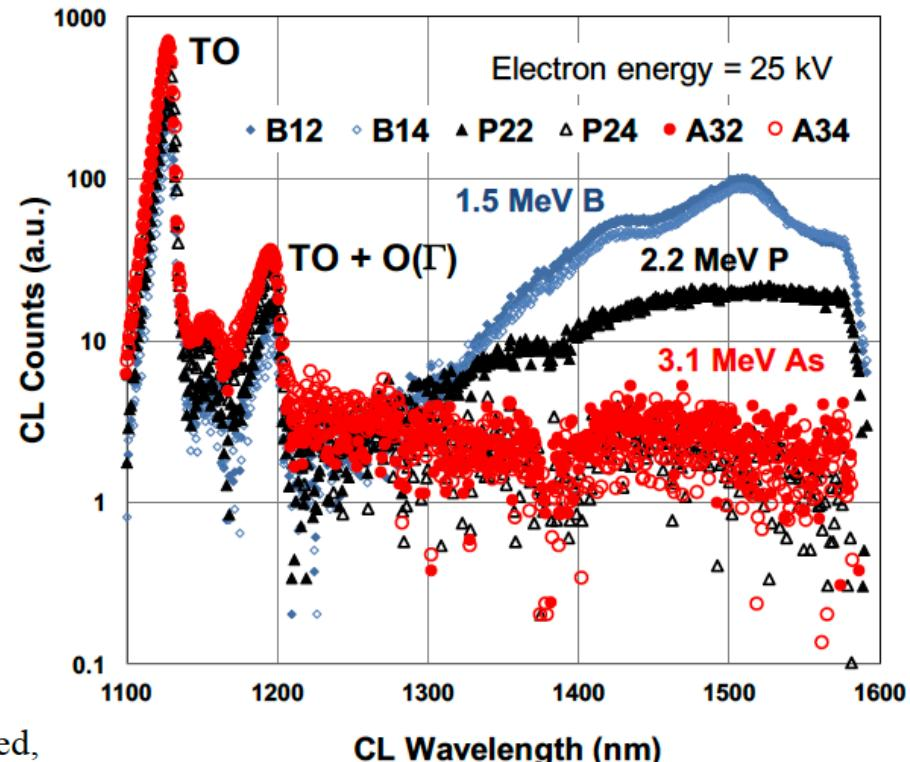
Fig. 17. CL recombination spectra (at 35 K) for annealed, highly-channeled implants into Si with 1.5 MeV B (diamonds), 2.2 MeV P (triangles) and 3.1 MeV As (circles) with an electron probe beam energy of 25 kV. Implants at 25 C filled symbols, at 450 C open symbols. Defect-related recombination emission is in the range of 1350 to 1600 nm. Transverse optical emission (TO) peaks are emissions from phonon-assisted (non-defect) recombination from conduction to valance band.
