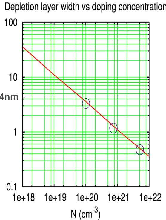
The Si body should be at least 4 nm thick @  $1 \cdot 10^{20}$  |e|/cm<sup>3</sup> To account for a proper depletion length
