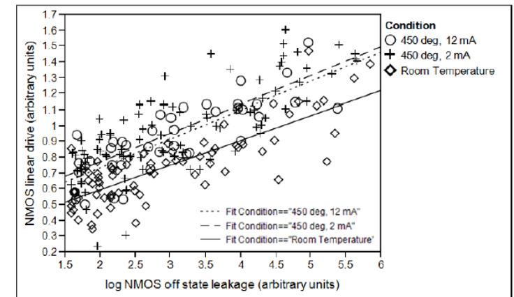
Fig. 5a: Trigate NMOS linear drive current plotted versus off state source-to-drain leakage for representative wafers at room temperature, 450 deg C at 12 mA beam current, and 450 deg C at 2 mA beam current
