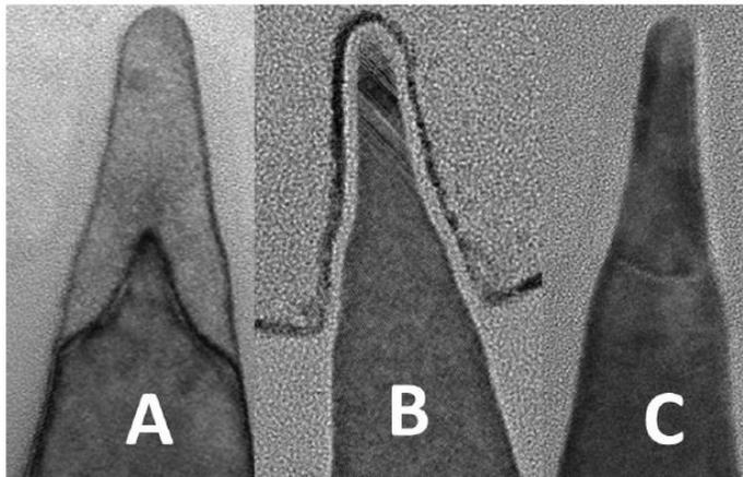
Fig. 1: TEM cross sections of silicon fins (A) immediately after room temperature implant, (B) after room temperature implant and a spike anneal (1 sec at  $\sim 1000^{\circ}\text{C}$ ), and (C) after heated implant alone (no anneal).
