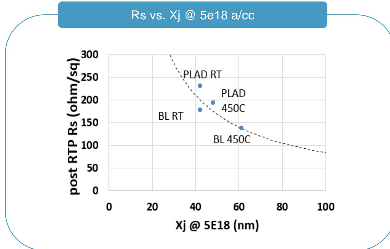
*Fundamental Implant Damage and Recovery Model Drives Implantation and PLAD to same Rs vs. Xj Curve
