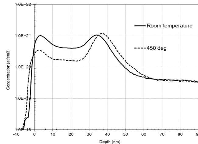
Fig. 3: SIMS profiles of 3.5 keV arsenic implanted at 30 degree incidence to wafer surface/fin top surface into fins nominally  $\sim 35$  nm tall with  $\sim 42$  nm pitch at room temperature and at 450 degrees.
