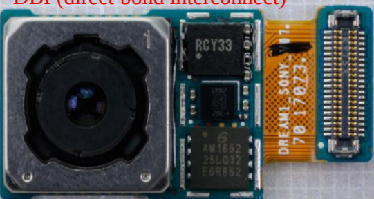
Sony 12Mp Rear facing Camera with DBI (direct bond interconnect)
