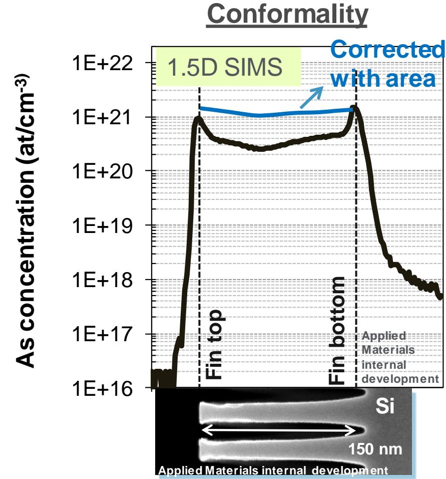
Plasma doping enables high doping concentration on surface and is a promising enabler for conformal contact
