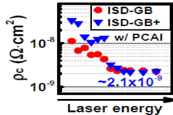
Optimization of Implant and nanosecond laser anneal resulted in  $\rho_c: \sim 2 \times 10^{-9} \Omega \cdot \text{cm}^2$
