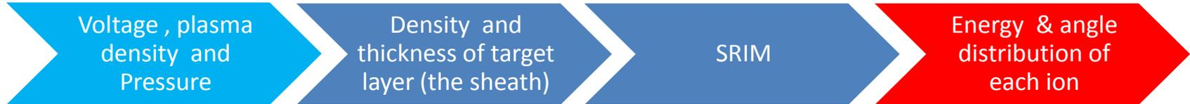
Example for AsH3 plasma : implantation of As at 500 eV through 1 mm of As gas
