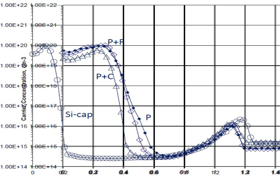
SRP for P-implant and co-implant in 1um Ge-epi wafers after 625°C RTA annealing
