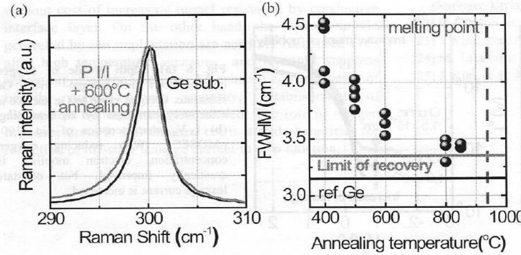
**Fig. 4** (a) Typical Ge Raman peaks (around 300  $\text{cm}^{-1}$ ) before and after P ion implantation with a dose of  $3 \times 10^{15} / \text{cm}^2$  and thermal annealing. (b) Annealing temperature dependence on crystallinity recovery of Ge. Although the annealing temperature was increased up to 850°C, still crystallinity is still worse than that of initial Ge substrate.
