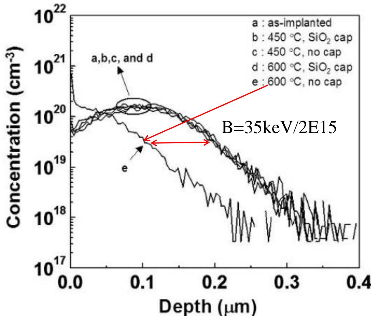
Fig. 4. SIMS profiles of ion-implanted boron in the Ge wafer with/without an  $\text{SiO}_2$  cap layer as a function of temperature.
