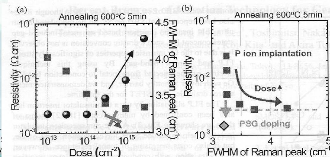
**Fig. 5** (a) Resistivity and FWHM of Raman peak of P implanted GeOI as a function of implantation dose. Above  $3 \times 10^{14} / \text{cm}^2$ , FWHM of Raman peak is increased and reduction of resistivity is saturated. (b) Correlation between resistivity and FWHM of Raman peak. By solid phase diffusion with phosphorous silicate glass (PSG), further reduction of resistivity is achieved without increasing FWHM of Raman peak.
