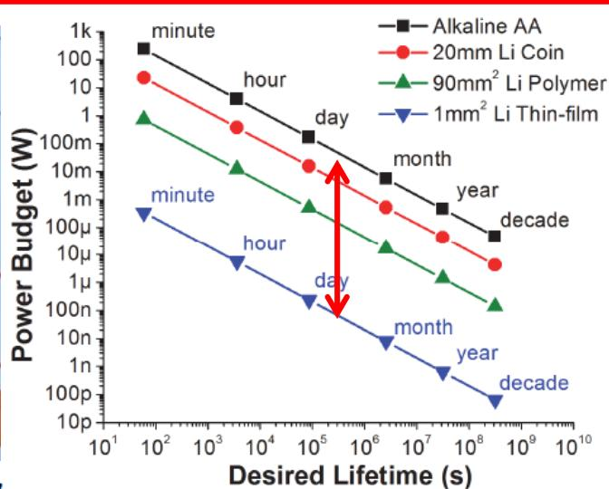
Figure 1. Average power draw constraint as a function of lifetime and battery size
