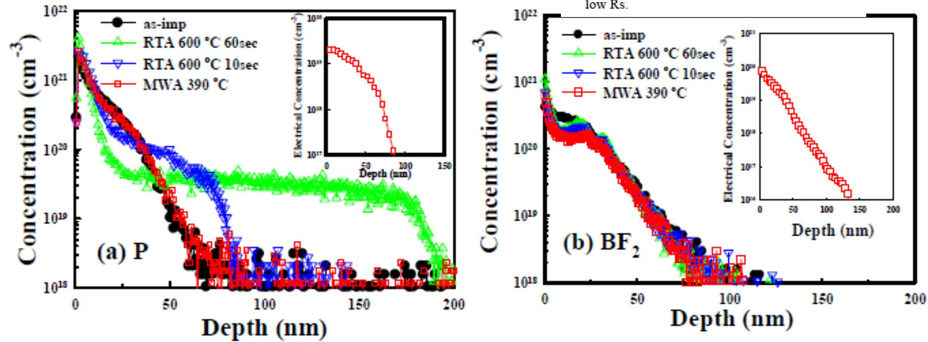
Fig. 3 SIMS and SRP profiles of (a) P and (b)  $\text{BF}_2$  at  $1 \times 10^{15} \text{ cm}^{-2}$  in (100) Ge. The P distribution after MWA is identical to as-implanted, but not after RTA. All boron distribution profiles are close to as-implanted. The insets show the activated levels of P and B by SRP are  $2 \times 10^{19} \text{ cm}^{-3}$  and  $7.5 \times 10^{19} \text{ cm}^{-3}$ .
