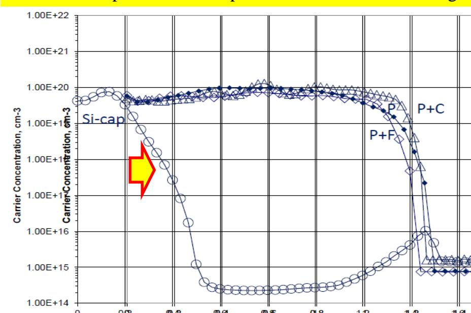
SRP for P-implant and co-implant in 1um Ge-epi wafers after 900°C RTA annealing
