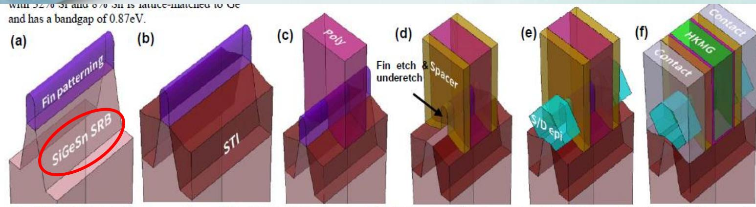
Fig. 3 MOSFET fabrication process flow (a) Fin, SiGeSn SRB patterning (b) STI formation (c) Poly gate definition (d) Spacer formation and S/D recess (e) *In-situ* doped S/D epitaxial re-growth (f) Gate last high-k metal gate.
