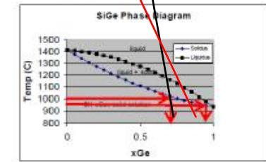
Figure 1. Binary phase diagram for Si-Ge. Note the continuous range of solid solutions for Si<sub>x</sub>Ge<sub>1-x</sub> alloys, which form random solid solutions in a diamond cubic structure.
