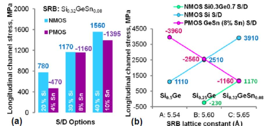
Fig. 12 Different options for tuning the channel stress: (a) Si content in NMOS S/D stressor, Sn content in PMOS S/D stressor (b) Lattice constant of the common SRB. Channel material kept invariant: GeSn (4% Sn) (PMOS) and Ge (NMOS), '7nm' design rules.
