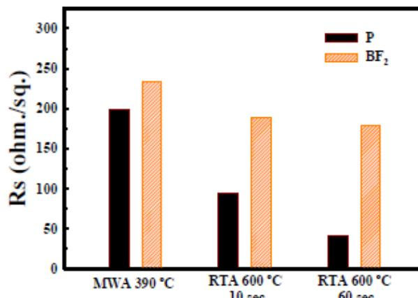
Fig. 4 The comparisons of the Rs between MWA and RTA in (100) Ge. The deep junction of P formed by RTA results in the low Rs.
