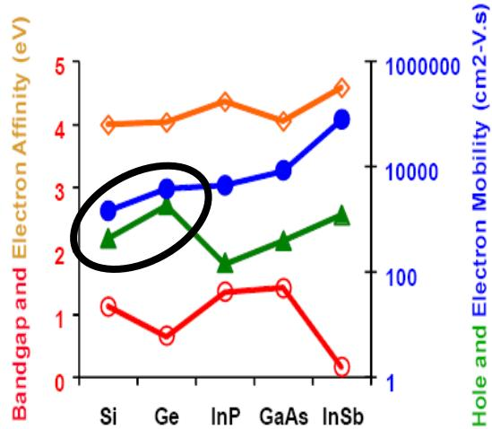
Figure 16. Key electronic parameters for major semiconductors.
