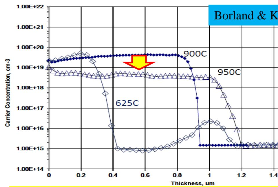
SRP for As-implant 1um Ge-epi wafers after RTA annealing
