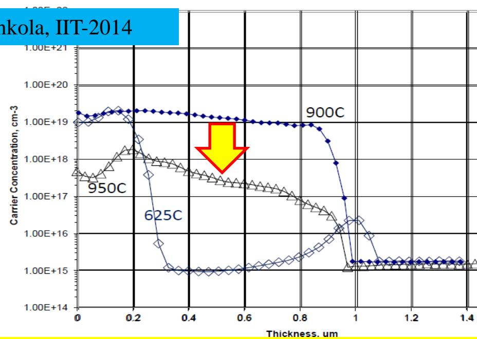
SRP for Sb-implant 1um Ge-epi wafers after RTA annealing
