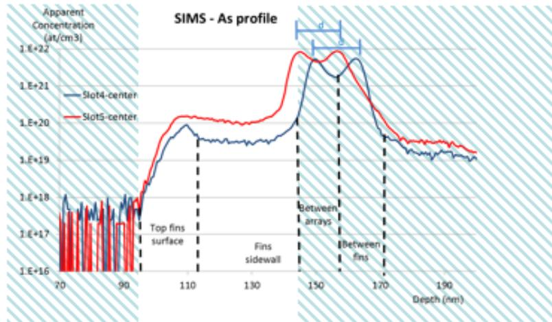
SIMS uses integral deconvolution to calculate As dose at fin top and fin sidewall.
