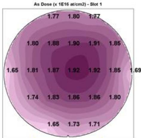
Good non uniformity of PULSION implantation on Fin structured wafers (Non unif < 3%)
