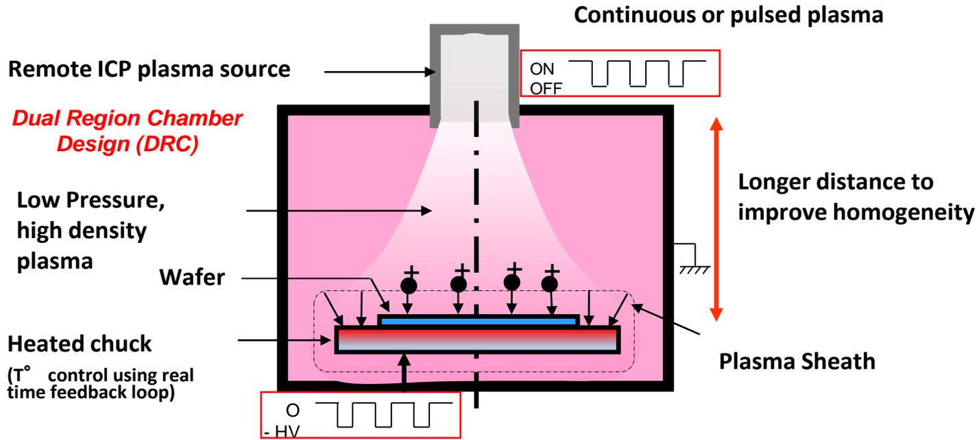
Schematic of PULSION® with high temp chuck option
