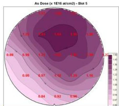
Dose loss and non uniformity if SiO<sub>2</sub> cap layer deposition & etch and annealing processes are not well controlled (Non unif = 15%)
