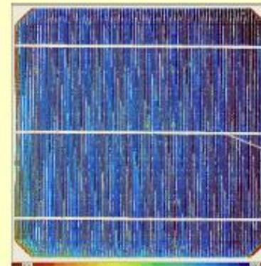
Map of Light Beam Induced Current of a 19.3% cell. Mean Diffusion Length ~700µm
