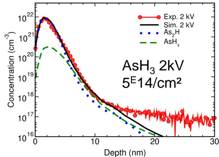
IIT2014 : Simulation of AsH<sub>3</sub> Plasma Immersion Ion Implantation into Silicon
