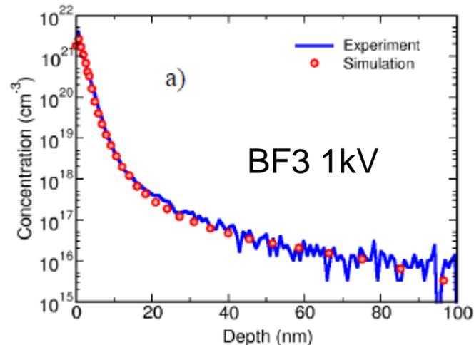
IIT2012 : Simulation of BF<sub>3</sub> Plasma Immersion Ion Implantation into Silicon
