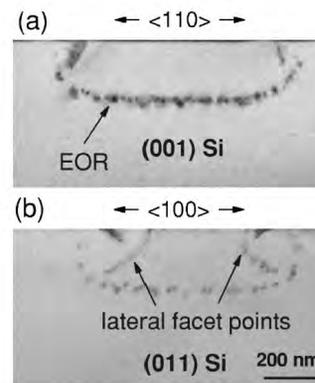
FIG. 7. Cross-sectional TEM images of (110)-aligned a-Si lines in (a) (001) Si and (b) (011) Si after annealing at 900 °C for 6 min.
