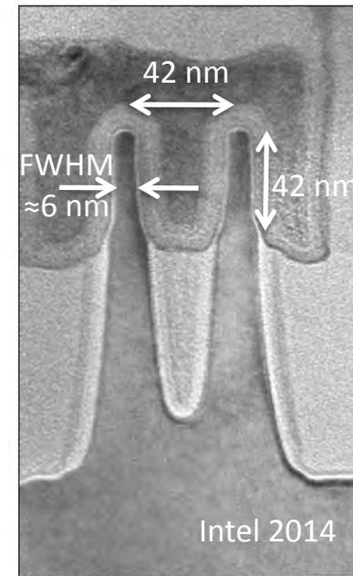
14 nm 2<sup>nd</sup> Generation Tri-gate Transistor
