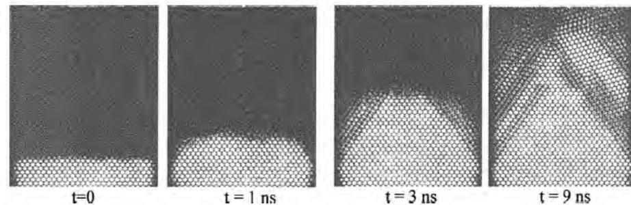
FIG. 6. Molecular dynamics simulations of the evolution of a 14 nm fin structure. A covering amorphous layer surrounds the Si fin. A crystalline seed is left at the bottom to promote solid-phase epitaxial regrowth. Poor regrowth causes {111} twin boundaries and polycrystalline Si.
