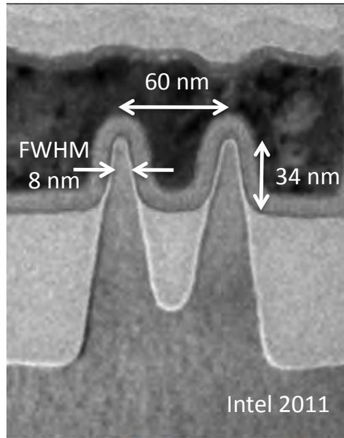
22 nm 1<sup>st</sup> Generation Tri-gate Transistor
