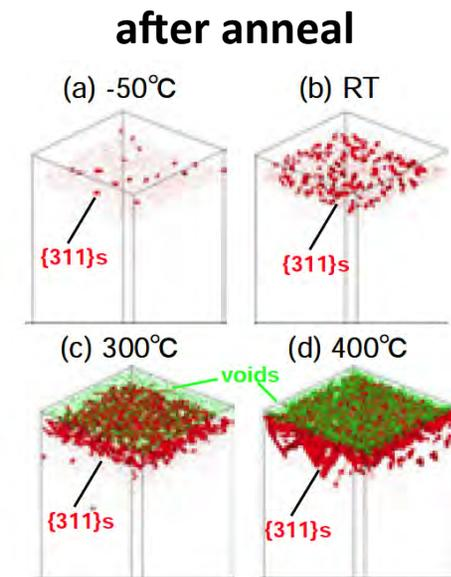
Fig. 4. KMC simulations of defects for As 5keV implant and low temperature SPER with different implant temperatures, (a) -50 °C, (b) Room Temperature (RT), (c) 300 °C, and (d) 400 °C, respectively. As implant temperature is increased, residual {311} defects are increased and elongated. Void (vacancy clusters) is also increased at high implant temperature. Noda IEDM13
