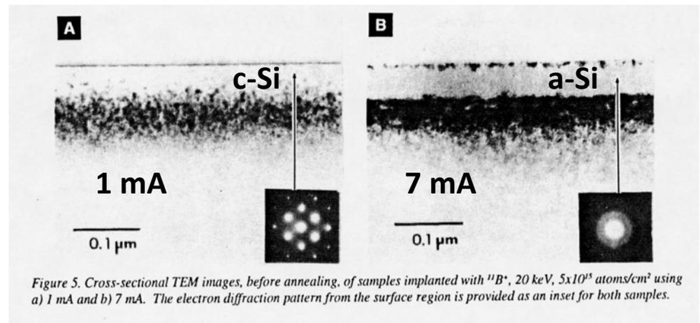
Figure 5. Cross-sectional TEM images, before annealing, of samples implanted with <sup>11</sup>B<sup>+</sup>, 20 keV,  $5 \times 10^{15}$  atoms/cm<sup>2</sup> using a) 1 mA and b) 7 mA. The electron diffraction pattern from the surface region is provided as an inset for both samples.
