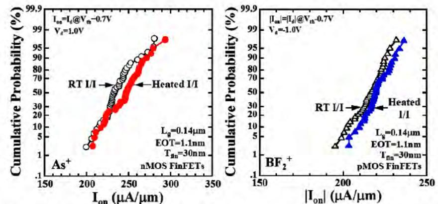
**Fig. 13** Ion distribution in nMOS and pMOS FinFETs processed by room temperature or heated ion implantation. Onoda IWJT14
