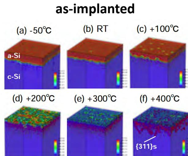
Fig. 3. KMC simulations for As 5keV implant with 6 different implant temperatures, (a) -50 °C, (b) Room Temperature (RT), (c) 100 °C, (d) 200 °C, (e) 300 °C, and (f) 400 °C, respectively. As implant temperature is increased, the depth of the amorphous-Si layer is reduced. {311} defects are formed during implant at higher implant temperature.
