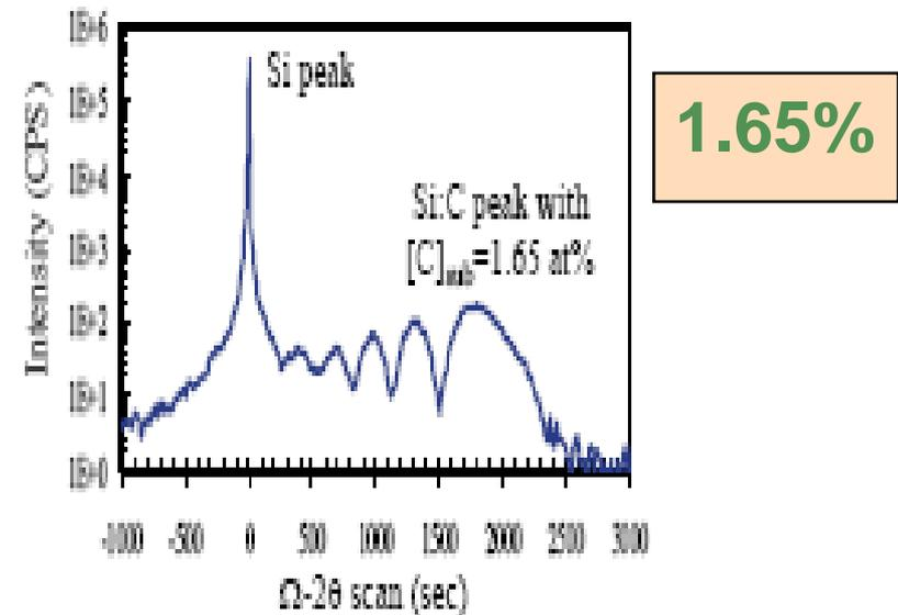
Fig. 2 HRXRD rocking curve of the SPE Si:C film ([C]<sub>sub</sub>=1.65 at%) grown on (100) Si substrate. The well defined Si:C peak and fringes indicate that the Si:C film is high-quality single crystal.
