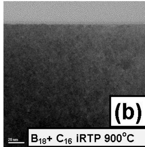
With diffusionless anneal, no EOR defects with  $B_{18}H_{22}$  and  $B_{18}H_{22} + C_{16}H_{10}$ .
