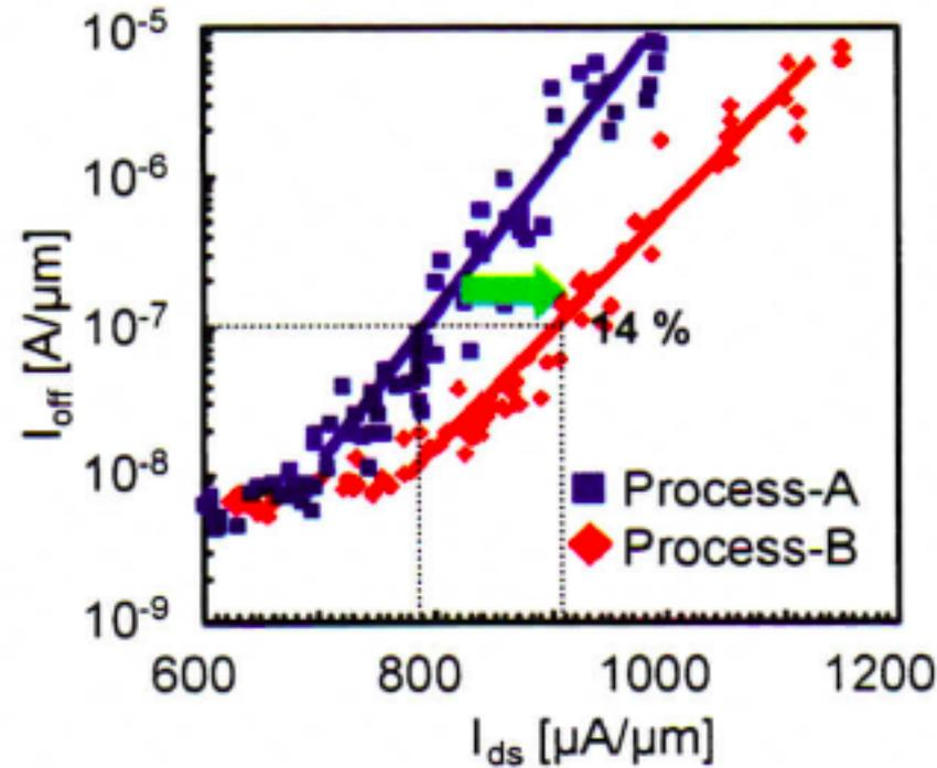
Fig. 10.  $I_{ds}$ - $I_{off}$  characteristics of nMOSFETs with Si:C-S/D using process-A and -B.
