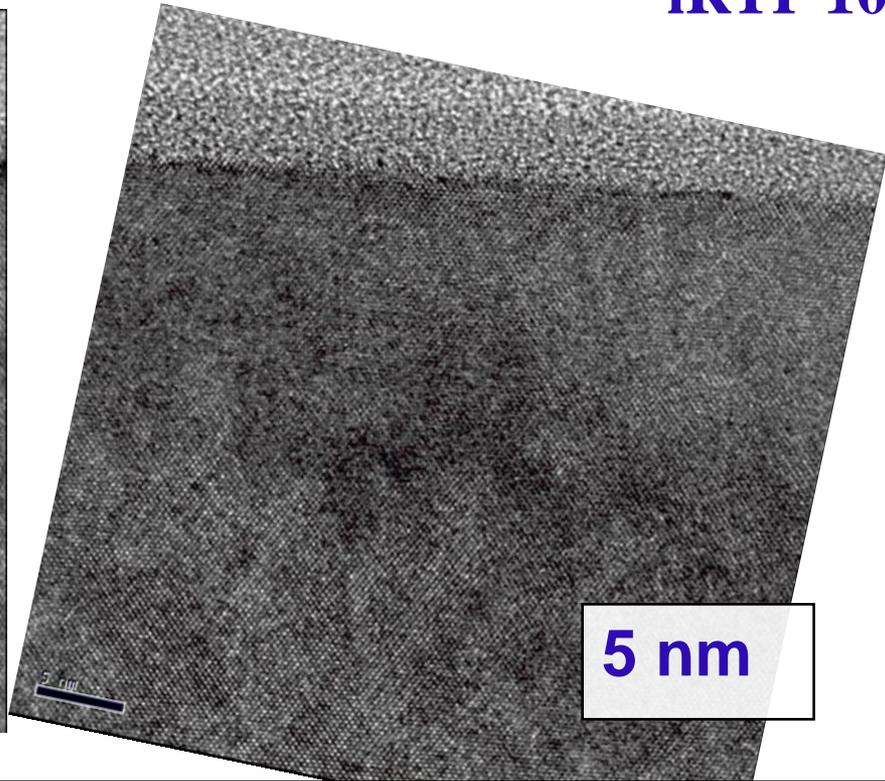
**No regrowth defects after iRTP 1050°C for both C<sub>7</sub> and P<sub>2</sub>+C<sub>7</sub> cases.**
