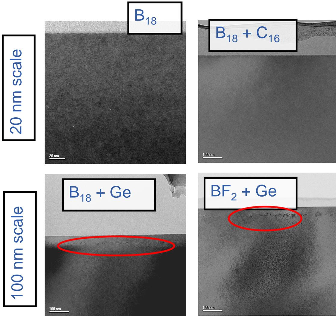
Ge co-implants produce EOR defects that remain following *iRTP @ 900°C*
