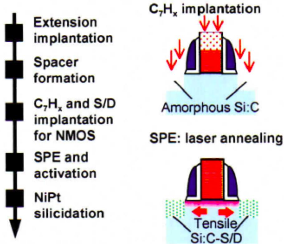
Fig. 1. Process flow of Si:C-S/D formation in nMOSFETs using C<sub>7</sub>H<sub>x</sub> implantation.
