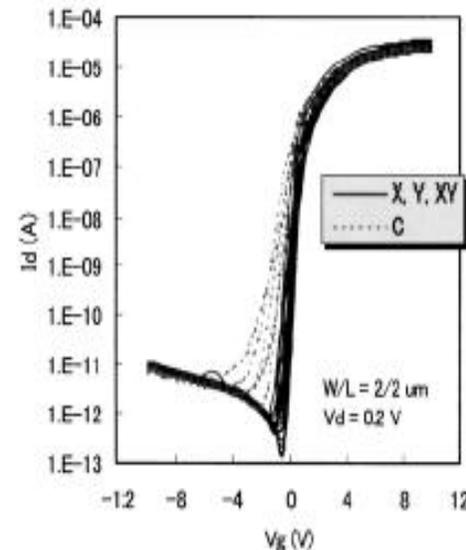
Fig. 3.  $I_d$ - $V_g$  characteristics of c-Si
