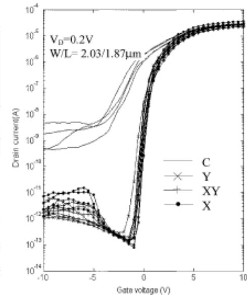
Fig. 2.  $I_D$ - $V_G$  characteristics of c-Si TFTs at various positions inside a grain-filter having ECR-PECVD  $\text{SiO}_2$  as a gate insulator
