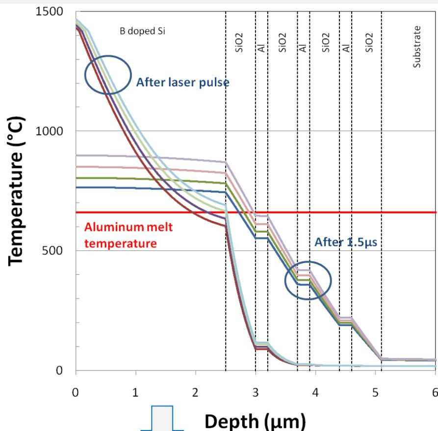
**Process Window determination to avoid damage of metal layer**
