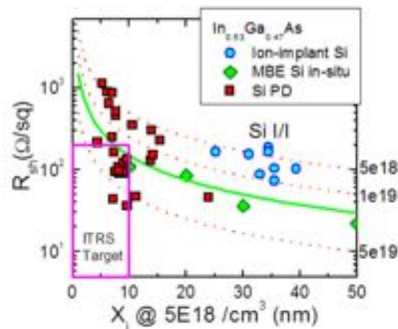
Figure of merit for junction doping in  $\text{In}_{0.53}\text{Ga}_{0.47}\text{As}$ . Si plasma doping results in significantly shallower junction depth and higher dopant incorporation compared to ion-implantation and in-situ doping technique. Green lines shows the focus of in-situ doping of Si during InGaAs epi deposition.
