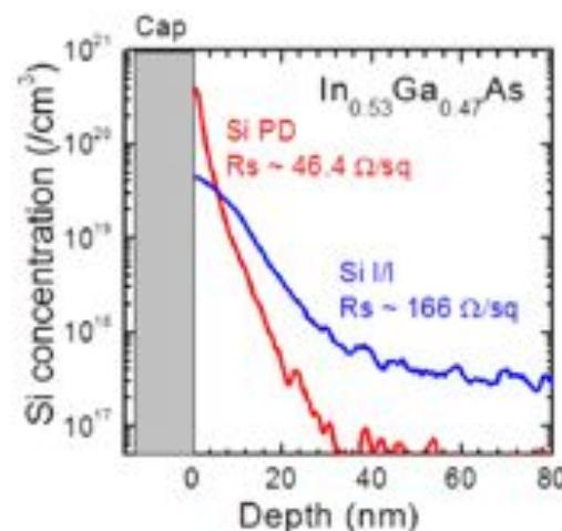
SIMS profile of Si in InGaAs introduced via Si plasma doping and conventional ion-implantation. Si plasma doping results in very steep abrupt profile with low background doping compared to ion-implantation.
