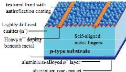
Figure 4: Schematic of the simplified PLUTO solar cell with screen-printed and fired rear aluminum contact and front metal lines only 20-25 microns wide.
