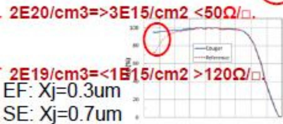
Figure 1: Typical internal quantum efficiency (IQE) curves for the Cougar selective emitter structure and a reference homogeneous emitter cell.
