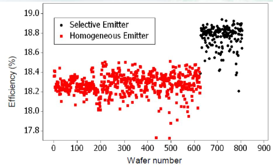
Fig. 9. Scatter plot of the conversion efficiencies (%) of selective emitter vs homogeneous emitter.
