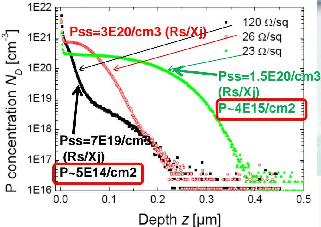
Figure 4: SIMS Profiles of the selective laser doped areas. For comparison, the shallow emitter with a sheet resistance of  $120 \Omega/\text{sq}$  emitter is also included.
