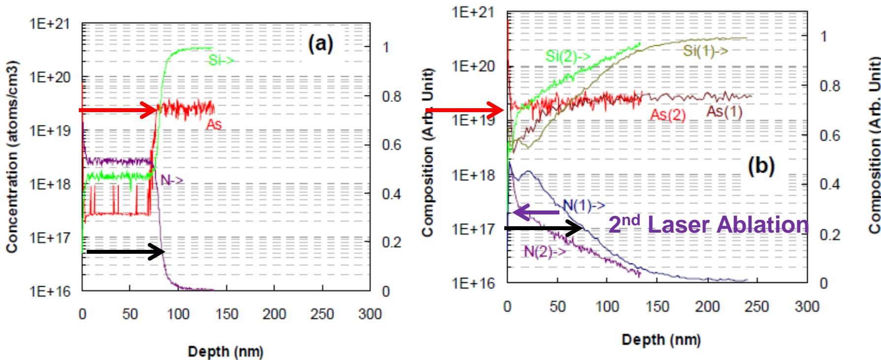
Fig. 6. SIMS element analyses at the area without holes (a), or at the area with holes drilled by one or two laser pulses (b).
