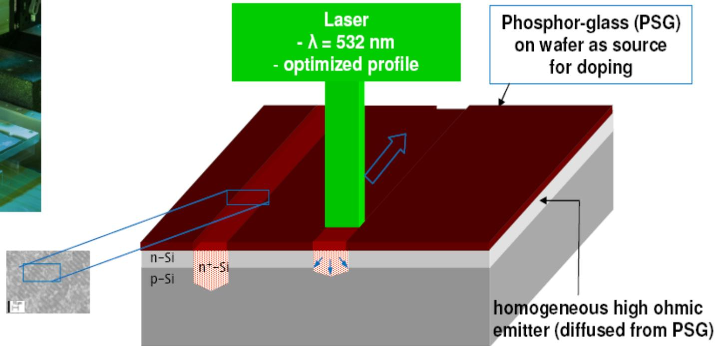
Only one laser process step added to mainstream cell process.
