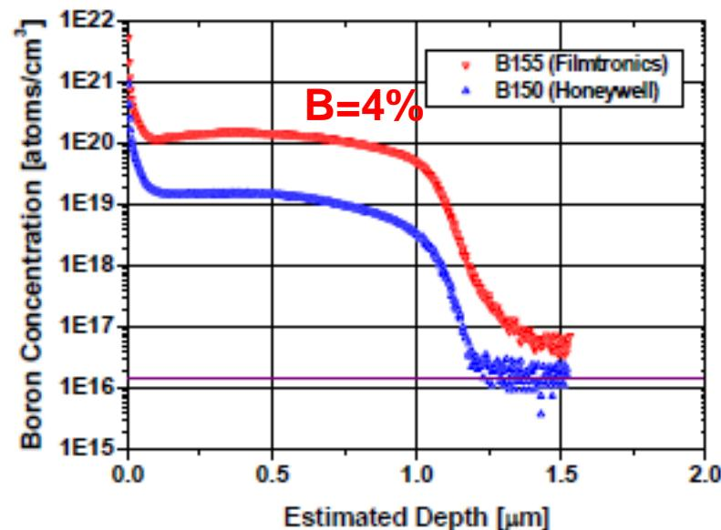
**Figure 2:** SIMS measurements of two different boron SODs. The solid line represents the background boron level of the substrate.
