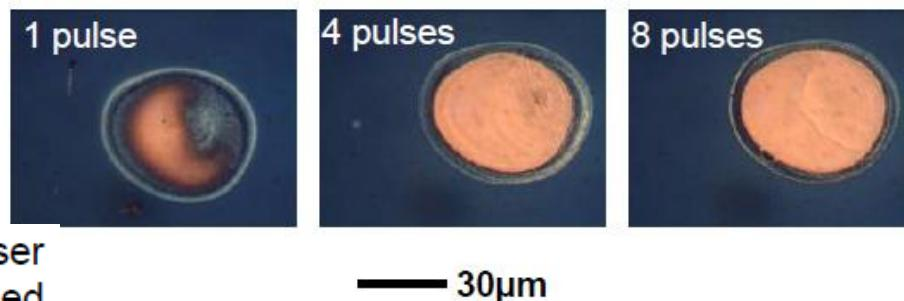
Fig. 5. Micrographs of laser drilled holes with different pulses used.
