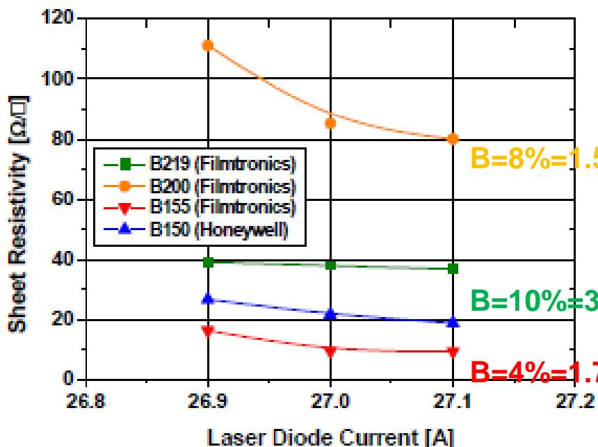
**Figure 1:** Sheet resistivity as a function of laser diode current for the four boron SODs. Solid lines are given as a guide for the eye.
