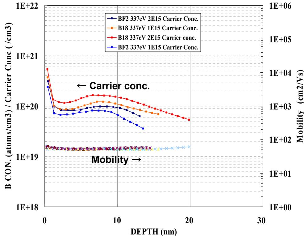
✓ The B18 cluster implants generate twice the activated boron for the same dose than the BF2 beamline implant does.
