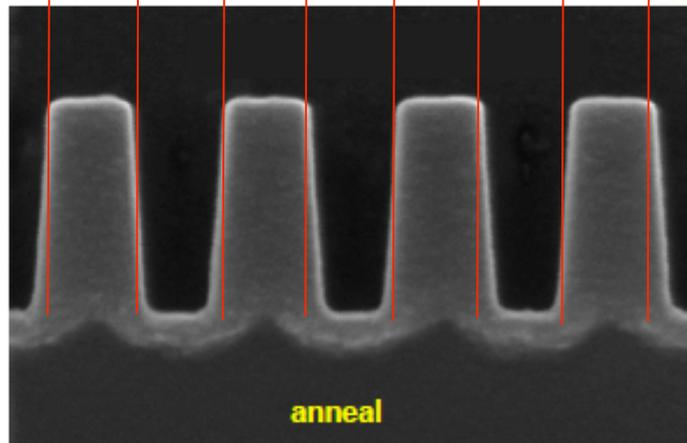
■ White layer is inside fin Si, since no change in fin dimensions and bright, white layer disappears in annealed sample
