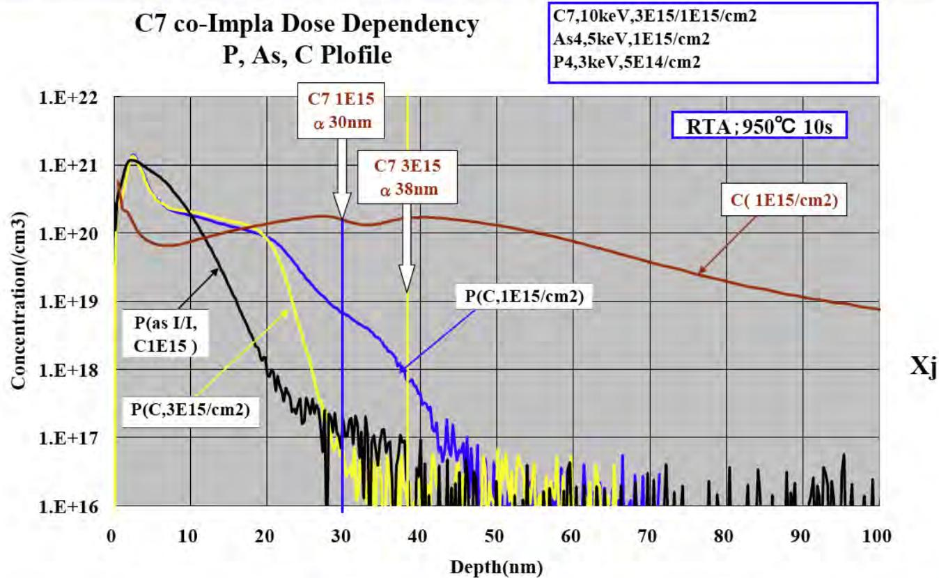
**To make a boxlike profile, carbon α layer should cover the P EORD area.**
