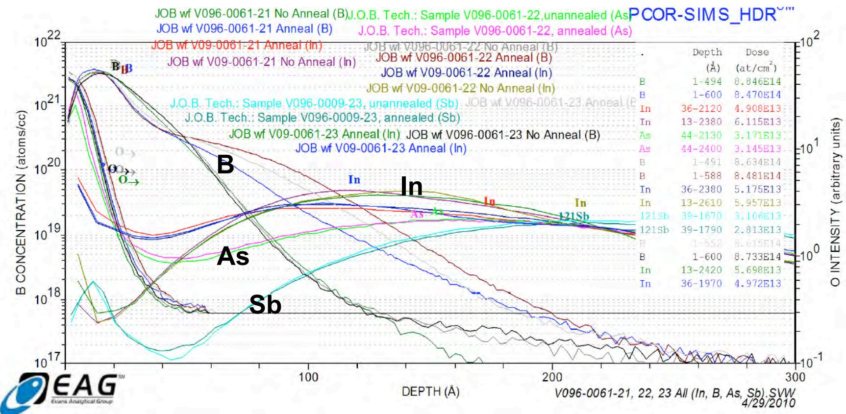
Note: In levels higher than As or Sb for <20 nm. Counter-doping?
