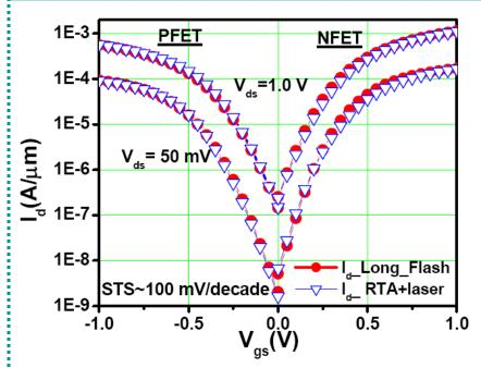
Long ms-flash implemented in a SOI process with a Poly/SiON gate stack was compared with a "combo process" of Spike-RTA + Laser Anneal
