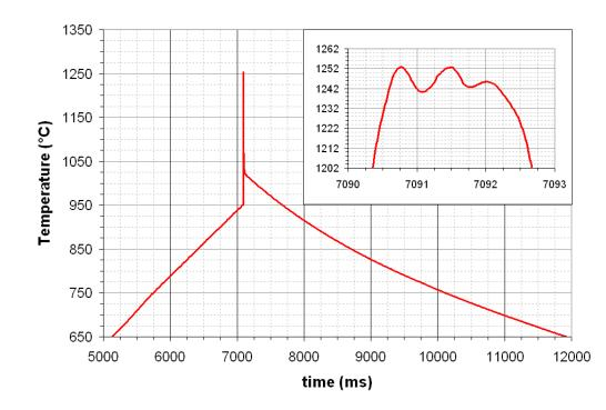
■ Real time control of lamps in Millios<sup>™</sup> allows for flat top temperate profiles
