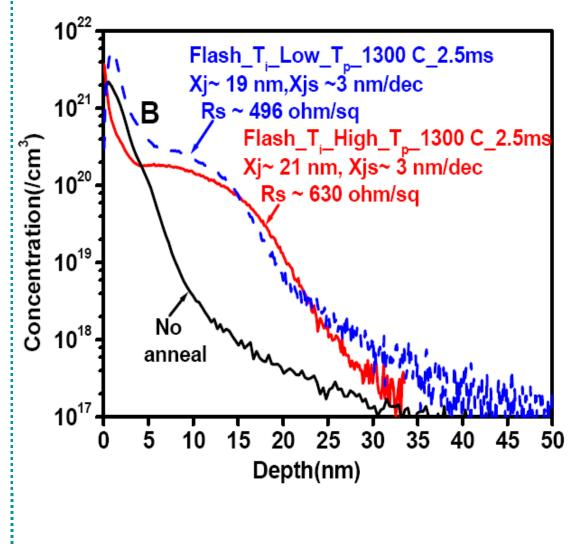
Using higher BF<sub>2</sub> I/I energy & dose, and an absorber on blanket I/I wafer to simulate device wafer reflectivity, long msflash with lower T<sub>i</sub> at T<sub>p</sub> of 1300°C was enabled and compared to one with higher T<sub>i</sub>
