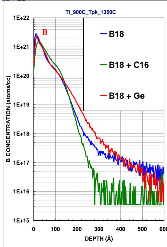
High boron concentration at Ge EOR defect region. Reduced concentration with  $C_{16}H_{10}$  at iRTP 900°C. The concentration is removed at the higher flash temperature  $T_{pk} = 1350^\circ C$ .
