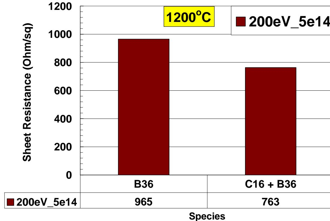
Using  $B_{36}$  or  $C_{16} + B_{36}$  one can get to low sheet resistance with millisecond anneal with  $X_j < 10\text{nm}$
