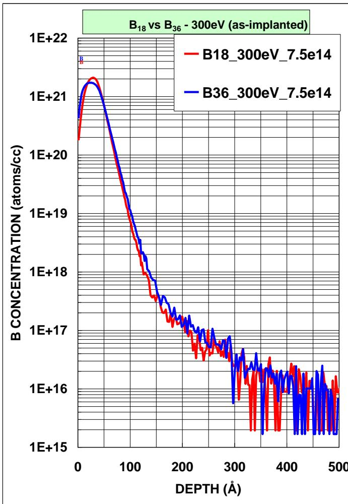
SIMS profile for B<sub>36</sub> is slightly deeper than B<sub>18</sub>. At a boron concentration of 5e18 atoms/cm<sup>3</sup>, the difference in Xj between B<sub>18</sub> and B<sub>36</sub> is around 5Å.
