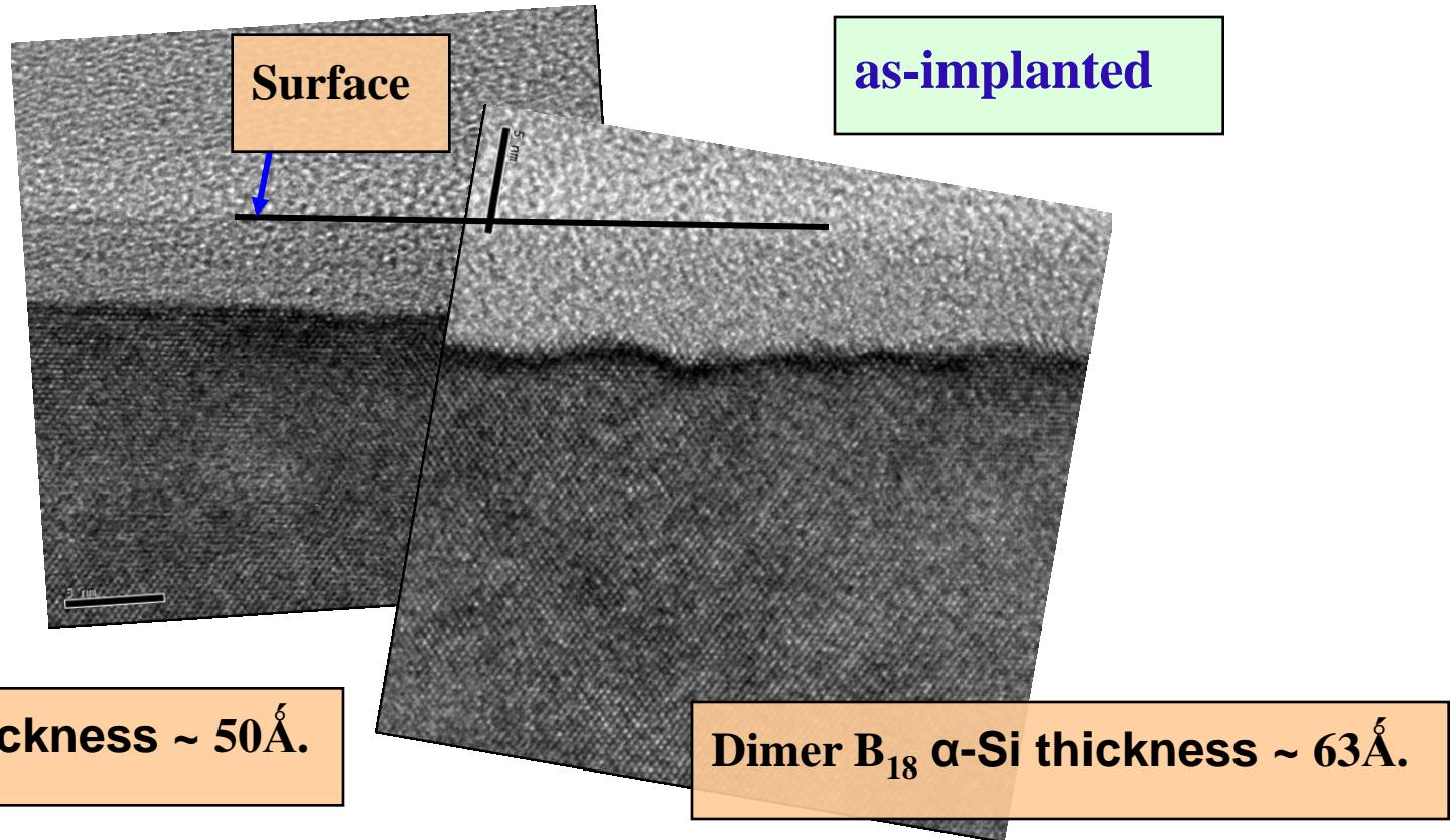
$B_{18}$   $\alpha$ -Si thickness  $\sim 50\text{\AA}$ .
