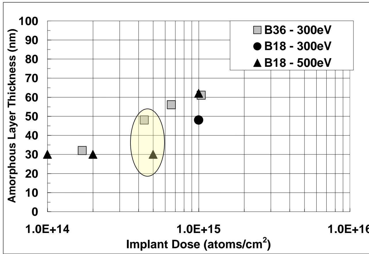
Amorphization threshold is lower with  $B_{36}$  compared to  $B_{18}$  even for  $E_{B36} < E_{B18}$
