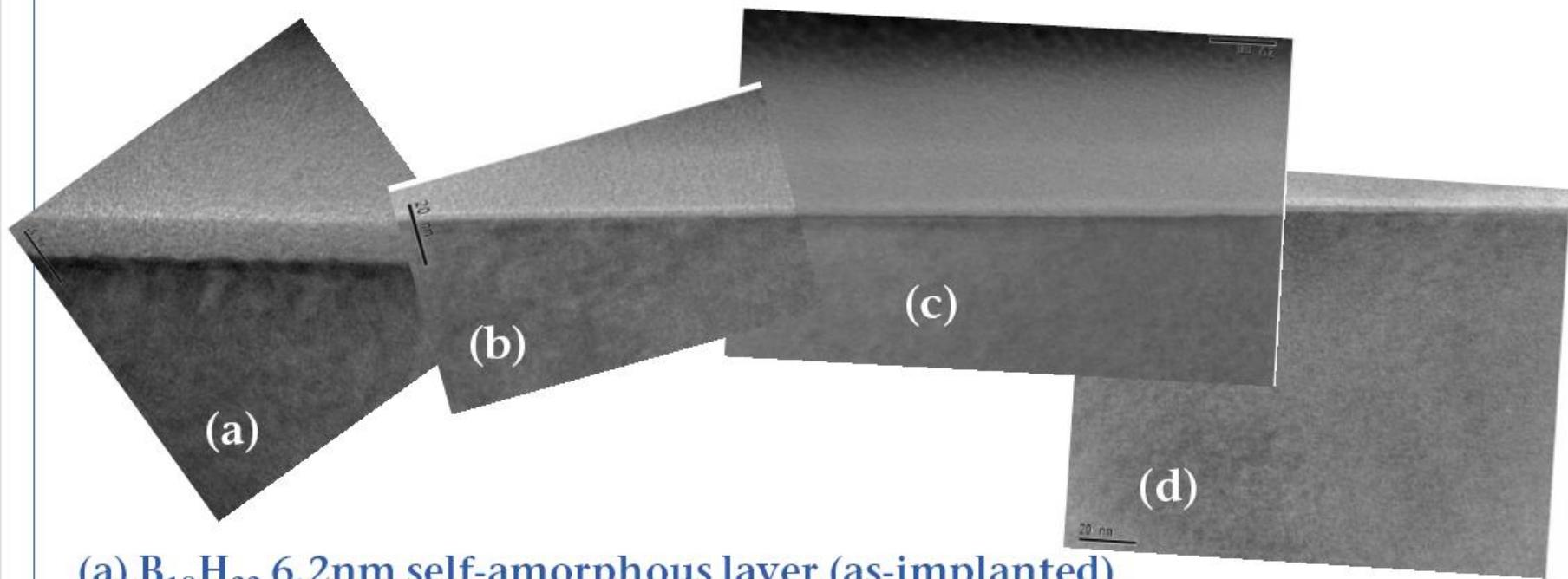
(a)  $B_{18}H_{22}$  6.2nm self-amorphous layer (as-implanted)
