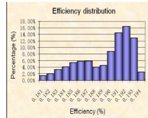
Figure 6: Typical efficiency distribution for a single-day's production of the 34MW PLUTO production line following 6 months of operation. The bi-modal distribution has been shown to be caused by wafers fitting into two distinct categories based on quality.
