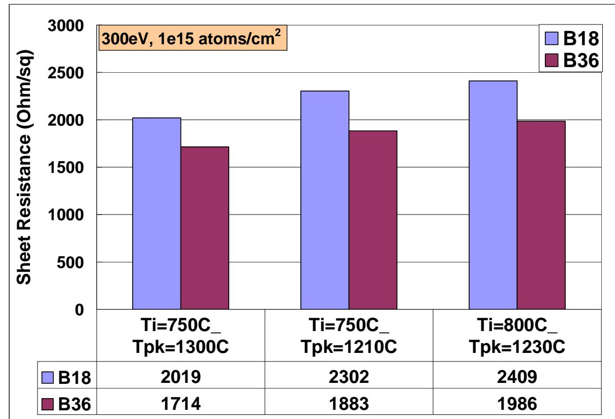
B<sub>36</sub> is better than B<sub>18</sub> by 15 – 20%. Possible explanation could be due to the higher amorphous layer thickness from B<sub>36</sub> implant.
