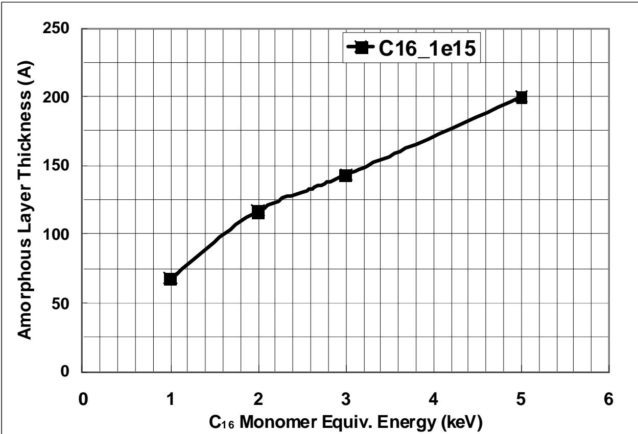
Provides a guidance to chose an energy and dose to obtain a given  $\alpha$ -Si thickness
