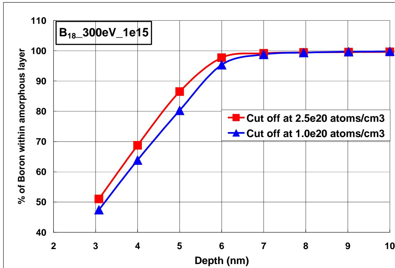
About 30% more boron is present in the  $\alpha$ -Si for a difference of 20 Å thickness in  $\alpha$ -Si (40 Å and 60 Å).
