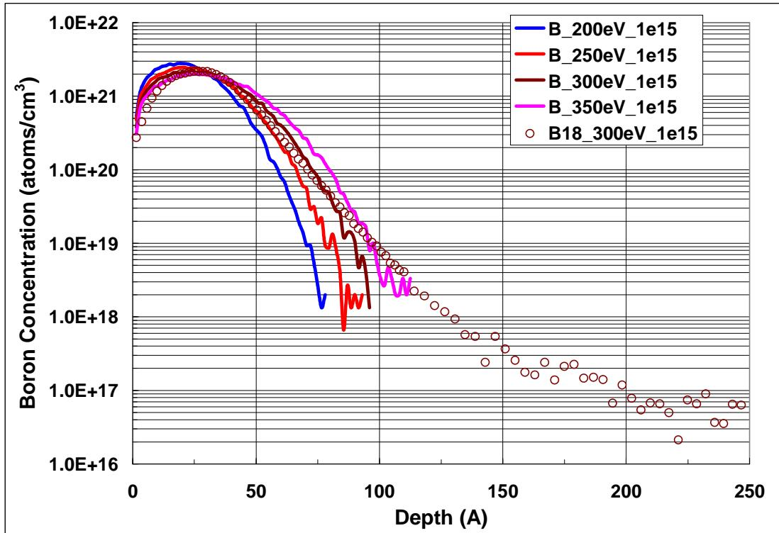
By choosing the right dose and energy Xj less than 10nm could be easily realized either with B<sub>18</sub> or Dimer B<sub>18</sub>.
