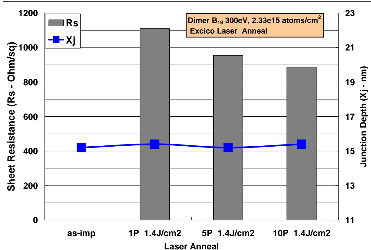
No change in Xj for various # of laser pulses at a laser energy density of 1.4J/cm<sup>2</sup>. But Rs lower by about 20% for 10 pulse case.
