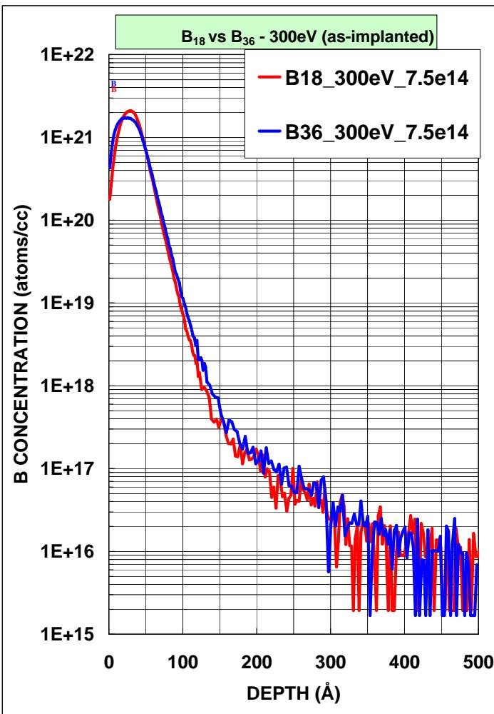
SIMS profile for B<sub>36</sub> is slightly deeper than B<sub>18</sub>. At a boron concentration of 5e18 atoms/cm<sup>3</sup>, the difference in X<sub>j</sub> between B<sub>18</sub> and B<sub>36</sub> is around 5Å.
