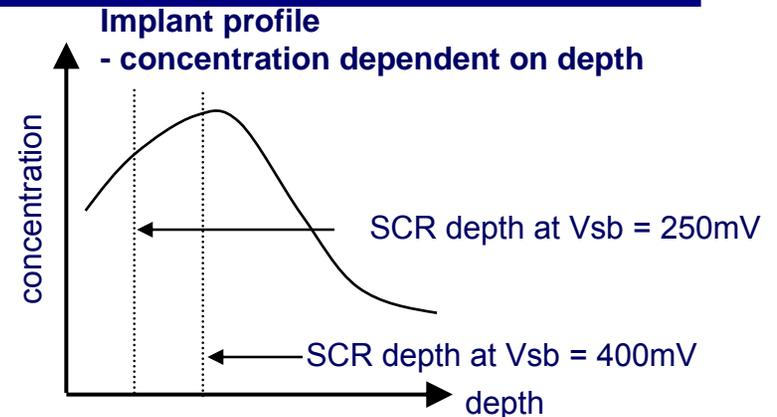
Measurement depth = Space Charge Region depth  $W$
