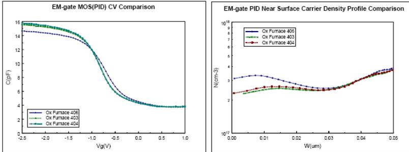
PID CV curve comparison of three oxidation furnaces. A clear distinction between furnace 403,404 and 406 can be seen. Furnace 406 shows a clear increase in carrier density by about 50% close to the surface.
