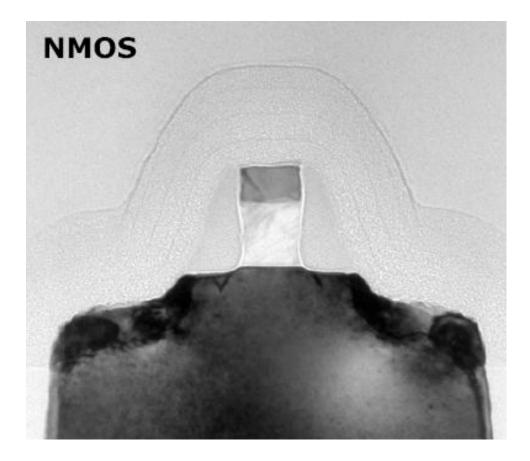
TEM image of a 42nm transistor from Intel's Presler chip, showing harmless dislocations under the spacers
