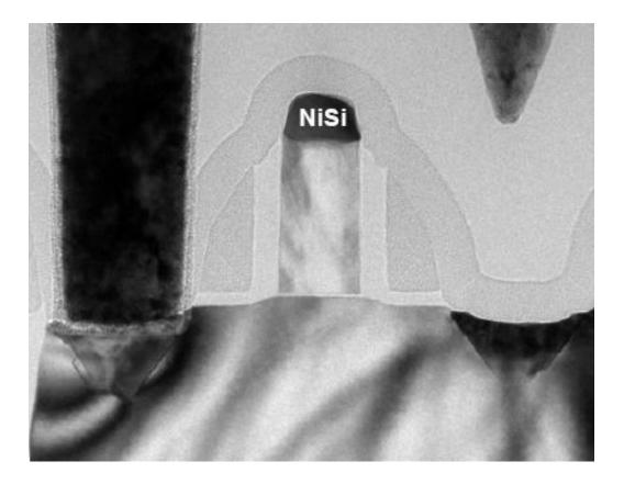
TEM image of a 55nm transistor from Matsushita's DVD SOC chip, showing dislocations under the silicide that are apparently harmless
