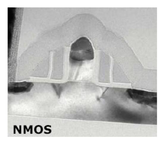
TEM image of a 50nm SOI transistor from AMD Athlon 64 2700 chip, showing harmless dislocations under the spacers
